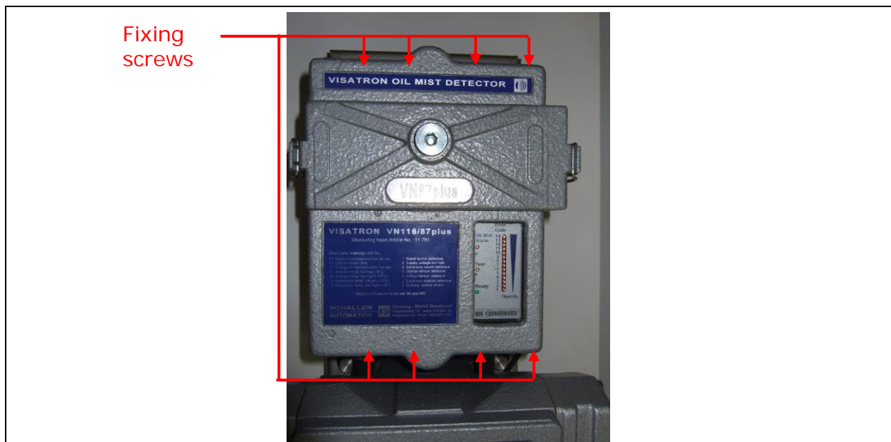
Figure 49: Step 3 is to unscrew the measuring head
