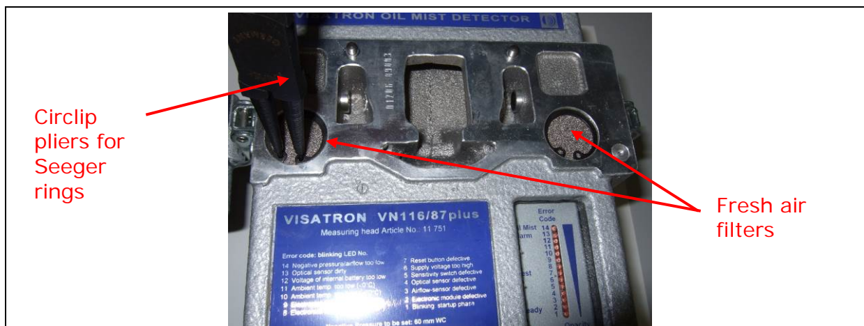
Figure 45: Exchange of the air filters
