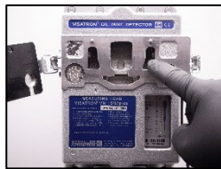
2. The infrared filter glasses may be dirty.
