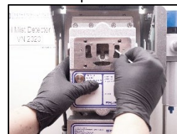
23. Clean the infrared sensor glass on the right side.
