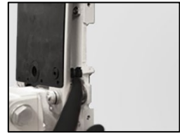
4. Check the flexible bellow for fresh air (Part no.: 10975). Replace if necessary!
