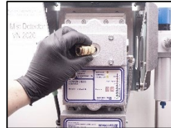
7. Install the quick connection.
