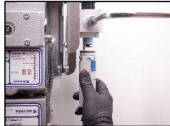
6. Reinstall the filter cage.
