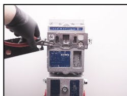
2. Replace the sintered bronze air filter/fresh air filter (part no.: 10042) and circlips (part no.: 10041).
