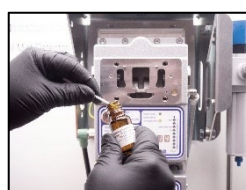
3. Use the cleaning fluid and cotton sticks.
