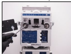
14. Change the scavenging air filter (Part nr.: 10042).
