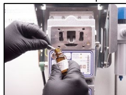
22. Use the cleaning liquid and cotton sticks.
