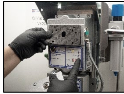
6. Clean the surface and replace the gasket for inspection cover.
