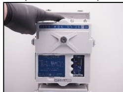
22. Check the heating element if it is hot. If cold – replace!
