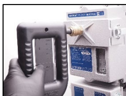
5. LED 14 will stop blinking, and the OMD will go back to ready.
