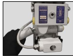
3. Reinstall the ejector input.
