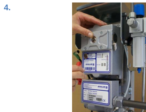
Figure 154: Loosen screws of the measuring head
