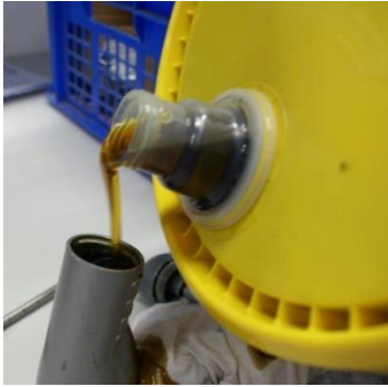
Figure 31: Fill lubrication oil into filling pump
