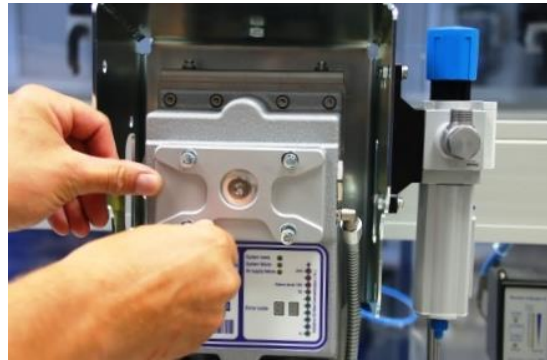
Figure 70: Fit the inspection cover
