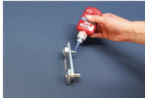
Figure 24: Screws with Loctite 243
