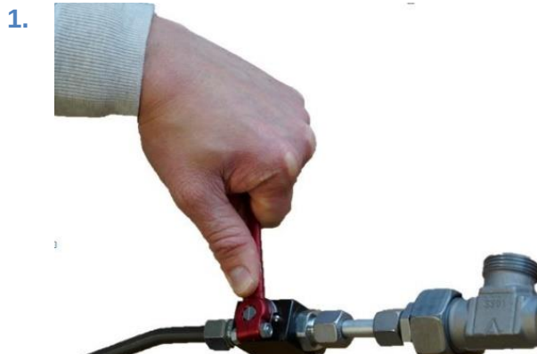
Figure 142: Switch off the compressed air supply
