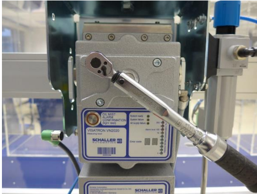
Figure 71: Tighten the inspection cover screws
