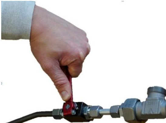
Figure 137: Switch off the compressed air supply
