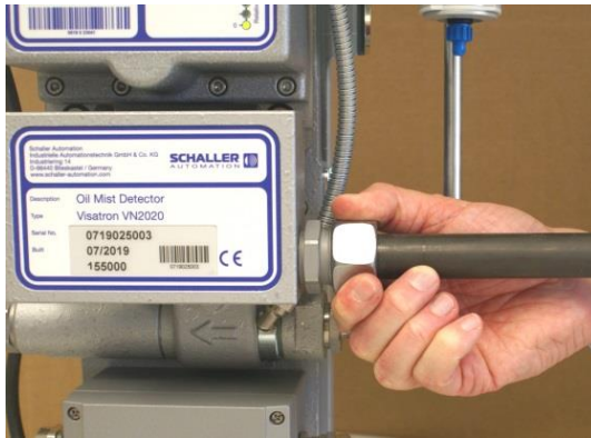
Figure 98: Fit the suction pipe
