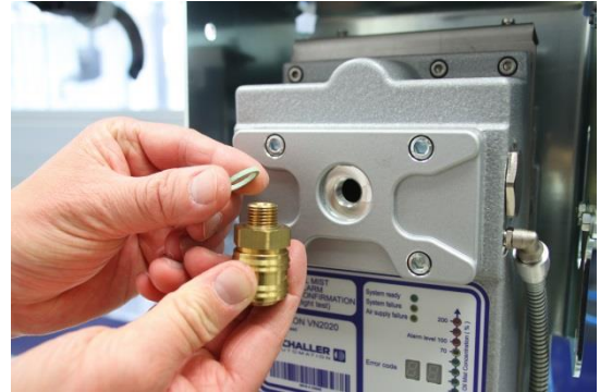
Figure 55: Inspection cover with quick-release coupling
