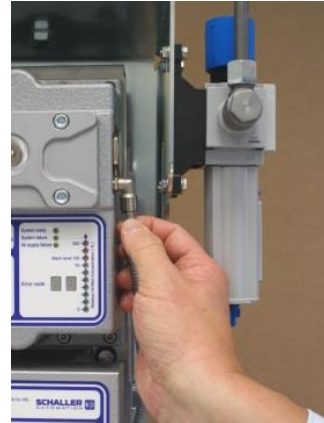
Figure 160: Fit the connecting hose
