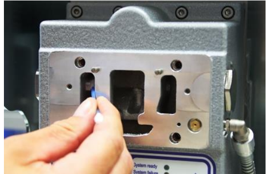
Figure 66: Clean transmitter diode
