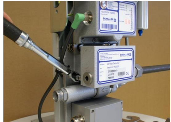
Figure 99: Tighten the connection box
