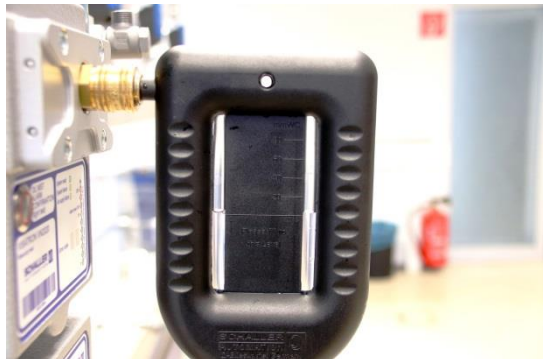
Figure 88: Check the negative pressure
