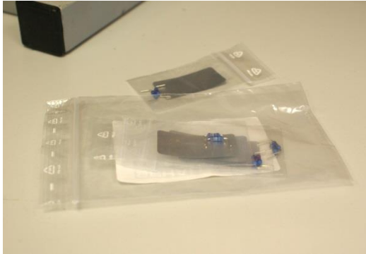
Figure 117: Remove the wire break resistors
