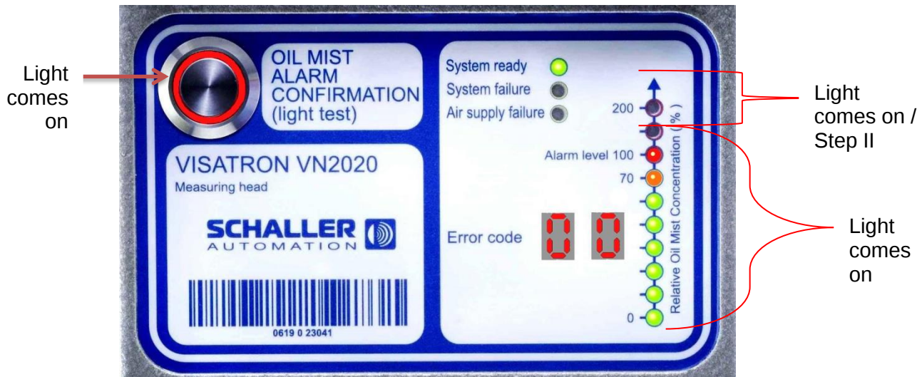
Figure 62: Example LED display with alarm
