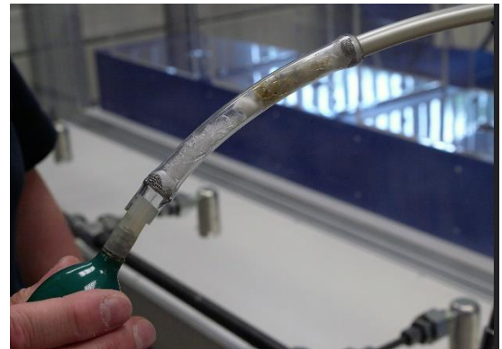
Figure 75: Connect the smoke tube and pump
