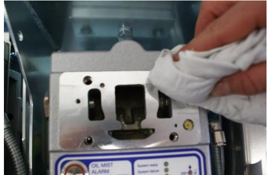
Figure 68: Clean sealing surface
