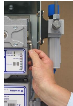
Figure 111: Fit the connecting hose
