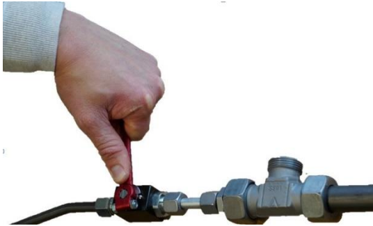
Figure 90: Switch off compressed air
