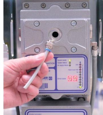
Figure 73: Fit the adapter hose
