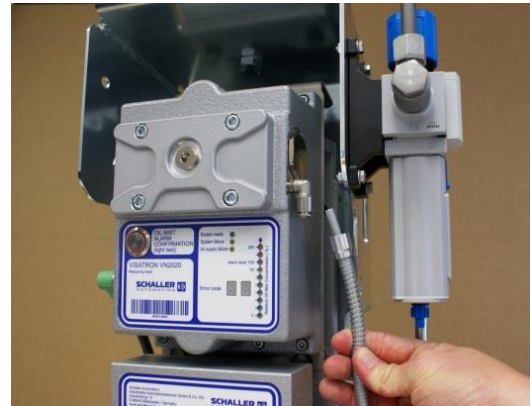
Figure 138: Remove the connecting hose
