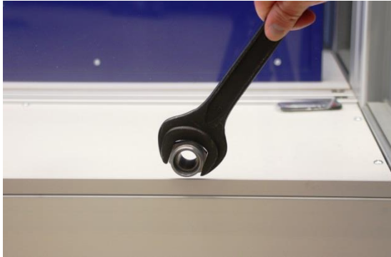
Figure 36: Mount screw-in socket
