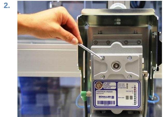
Figure 143: Loosen screw connection
