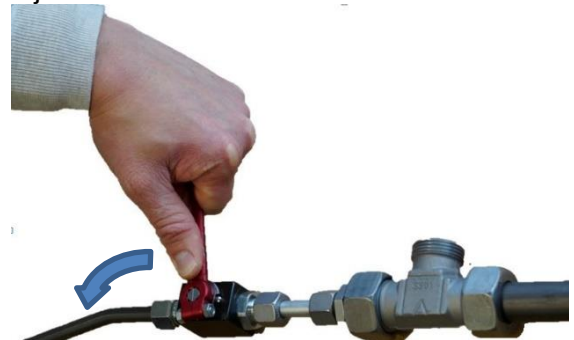
Figure 140: Switch on compressed air
