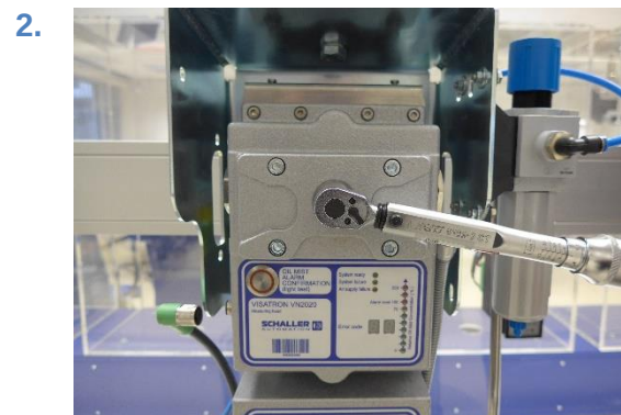
Figure 165: Screw in the screw plug
