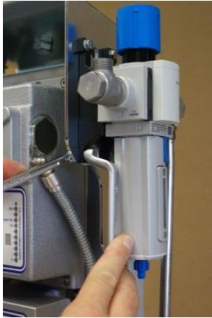
Figure 130: Disassemble the filter control valve
