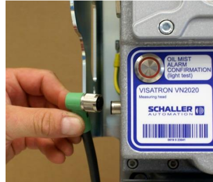
Figure 116: Unplug plug-in connector
