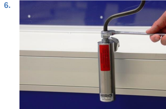
Figure 41: Tighten screw connection
