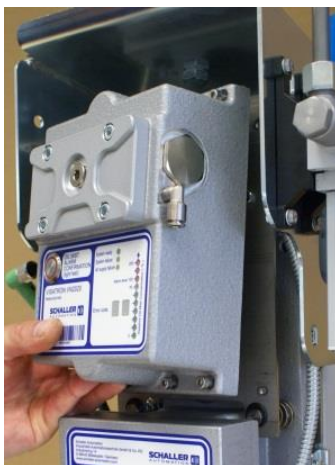
Figure 106: Remove the measuring head
