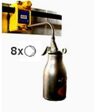
Figure 33: Pump lubrication oil
