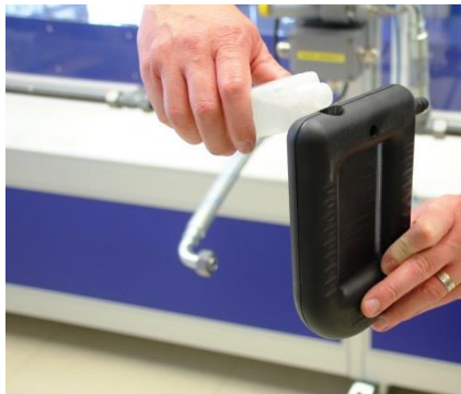
Figure 56: Fill U-tube manometer with water
