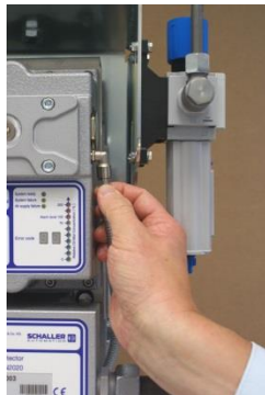
Figure 139: Fit the connecting hose
