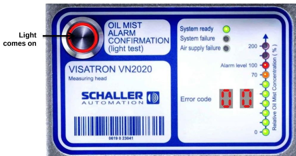
Figure 61: Display with detected oil mist
