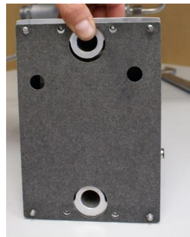
Figure 107: Place the mounting plate seal in position
