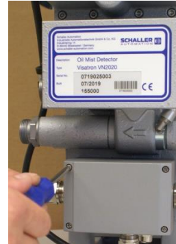
Figure 49: Install the cover of the terminal box
