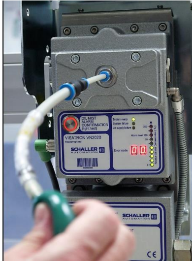
Figure 76: Pump smoke into the measuring head
