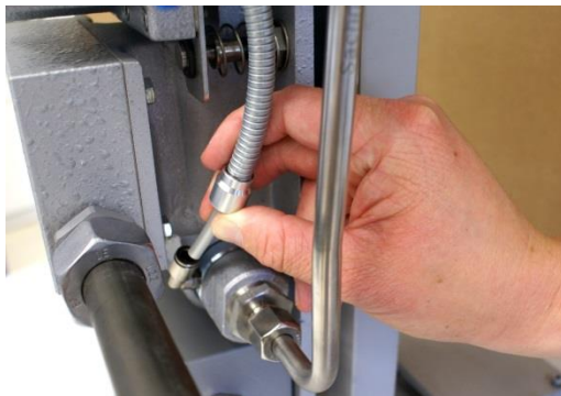
Figure 100: Fit the connecting hose
