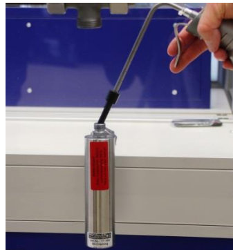
Figure 39: Fill the canister siphon
