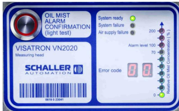
Figure 60: Measuring head display, in operating mode
