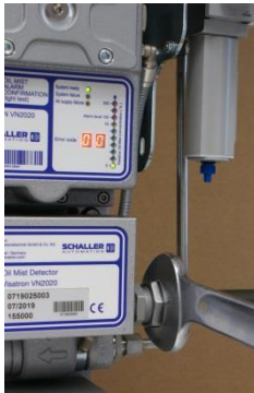
Figure 92: Loosen the screw connection
