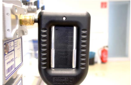
Figure 59: Negative pressure display on the U-tube manometer
