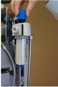
Figure 134: Release pressure in the filter control valve
