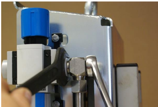
Figure 132: Tighten the swivel fitting
