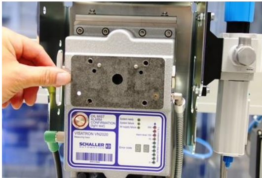
Figure 69: New inspection cover seal
