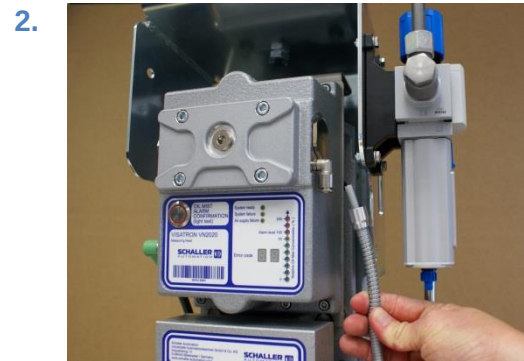
Figure 152: Remove the connecting hose
