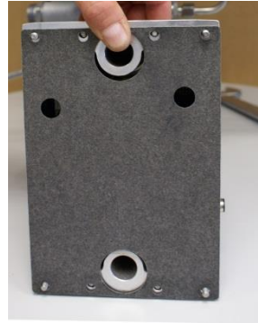
Figure 156: Place the seal in position
