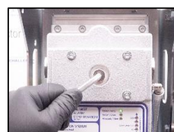
12. Disconnect the u-tube manometer and install the plug for inspection cover.
