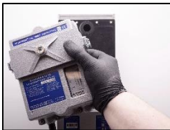
1. Replace the measuring head with an exchange unit.
