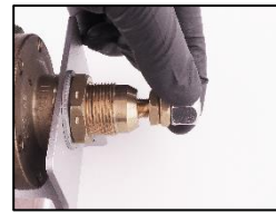
11. Adjust the air pressure to 55.00 – 65.00 mmWC!
