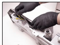
3. Disconnect the base plate from the connection cover.
