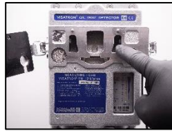
2. The infrared filter glasses may be dirty.
