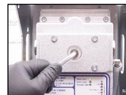
28. Remove the quick connection, and the oil mist detector is ready for operation!
