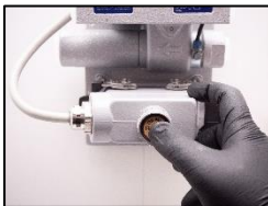
1. Press the RESET button several times.
