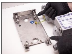
13. Check lower and upper measuring head suspensions for damage.
