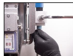
4. Unscrew the black plastic disc and remove the dirty filter.
