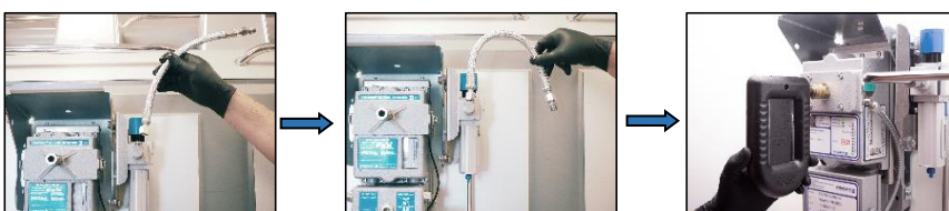
5. Finally connect the new pressure regulator to your air supply system with the new air supply hose and use a u-tube manometer to test and adjust the negative pressure to 55.00 – 65.00 mmWC!
