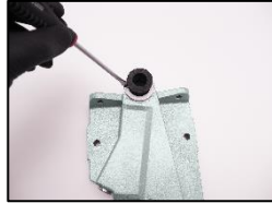
10. Replace the flexible bellows.
