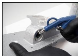
6. And into the ejector inlet and outlet chamber.
