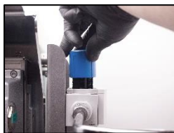
5. Adjust the air pressure to 55.00 – 65.00 mmWC!
