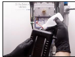
2. Fill in slacked water in the u-tube manometer.
