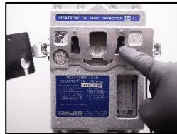
2. The infrared filter glasses may be dirty.
