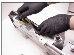
14. Replace the suspensions if necessary! Install the flexible damping plate back on the base plate.
