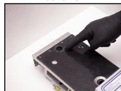
15. Ensure that position for the flexible bellow is correct.
