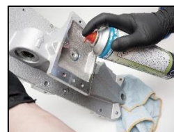
4. Clean the base plate for oil and dirt.
