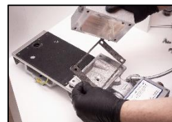
8. Replace the valve box gasket.
