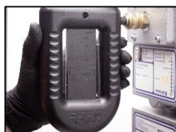
6. Connect the u-tube manometer and adjust the negative pressure to 55.00 – 65.00 mmWC!
