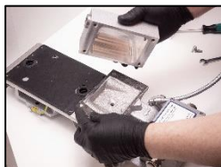
5. Replace the valve box gasket.
