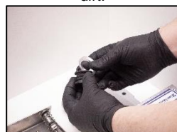
11. Check the upper bellow for damage, replace if necessary.
