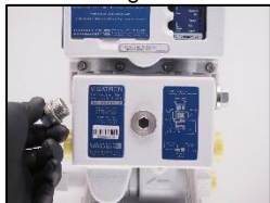
21. Change the screw plug seal 1/2".
