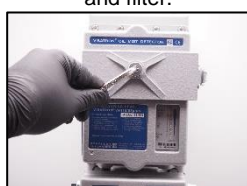
7. Turn on the air supply again and install the quick connection.
