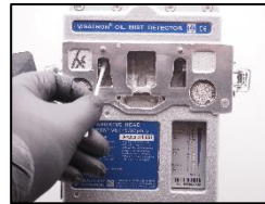
3. Clean the glasses with a cotton stick and technical alcohol.
