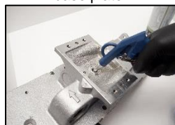
5. Use compressed air to the air channels into the base plate.
