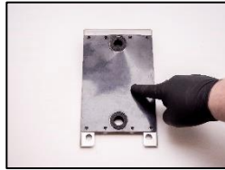
2. Check the measuring head gasket. If damaged, replace it.
