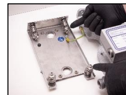
16. Check that grounding cable is connected at the flexible damping plate and the base plate.
