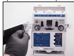
15. Change the seal for inspection cover.
