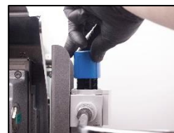
3. Adjust the air pressure to 55.00 – 65.00 mmWC!
