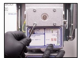
19. Unscrew the 4 pcs. bolts on the inspection cover.
