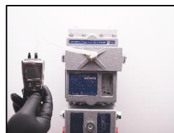
2. Connect the digital u-tube manometer to quick connection.
