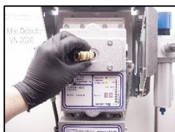
26. Connect the quick connection.
