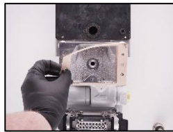
6. Change the valve box seal.
