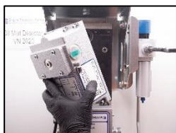
2. Disconnect the measuring head from the base plate.
