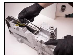
4. Loosen the bolts for pipe connection box.
