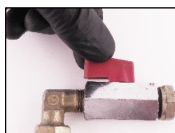
1. Turn off air supply to the oil mist detector.
