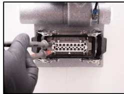
2. Measure supply voltage between pin 1 and 2 to be 18 and 31,2 V dc.
