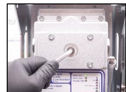
4. Disconnect the u-tube manometer and install the plug for inspection cover.
