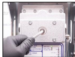
6. Disconnect the u-tube manometer and install the plug for inspection cover.
