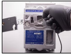
2. Use cleaning needle and clean the fresh air bores on the left and right side.
