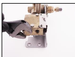
2. Unscrew the plug next to the air supply input.
