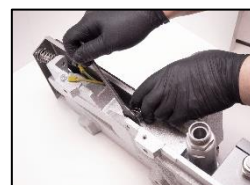
16. Reinstall the vibration damping plate.
