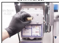
7. Install the quick connection.
