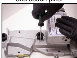
10. Disconnect the lower flexible bellow.
