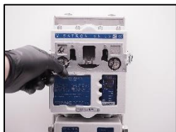
17. Clean the bores with cleaning needle.
