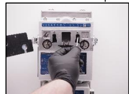
16. Clean the infrared sensor glasses with cotton sticks and cleaning fluid.
