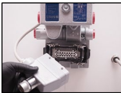
1. Remove the RESET task house.
