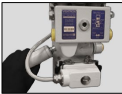
1. Disconnect the ejector input.
