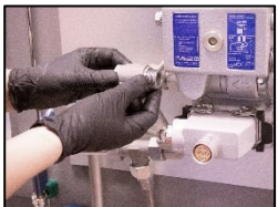
2. Remove the pipe from oil mist detector.
