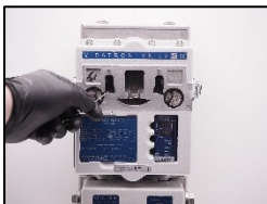
17. Clean the bores with cleaning needle (Part nr.: 10135).
