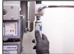
6. Reinstall the filter cage.
