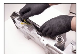
16. Reinstall the vibration damping plate.
