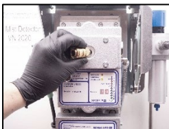
5. Connect the quick connection.
