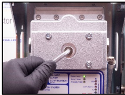
1. Remove the plug in the inspection cover.
