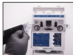
15. Change the seal for inspection cover (Part nr.: 11180).
