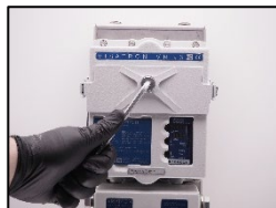
18. Change the screw plug seal ¼" for inspection cover (Part nr.: 10082).
