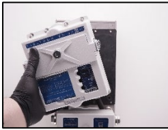
1. Remove the measuring head.
