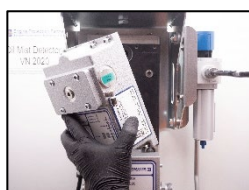
2. Remove the measuring head.
