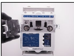
13. Open the inspection cover.
