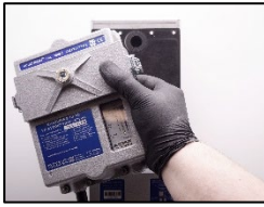
1. Remove the measuring head.
