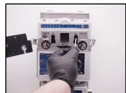
16. Clean the infrared sensor glasses with cotton sticks and alcohol (Part nr.: 10036 & 10035).
