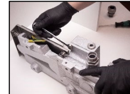
3. Unscrew the 4 pc. mounting bolts on the pipe connection box.
