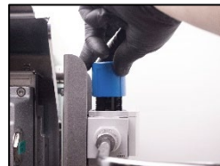
11. Adjust the air pressure to 60.00 mmWC!
