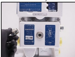
21. Change the screw plug seal ½" (Part nr.: 10209).
