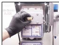
26. Connect the quick connection.
