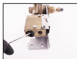
3. Use a small flat screwdriver to loosen the gasket, extract the gasket and filter.
