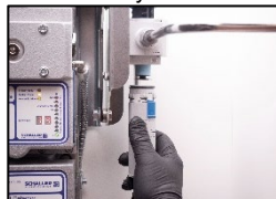
6. Reinstall the filter cage.
