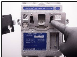
2. The infrared filter glasses may be dirty.
