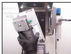
2. Remove the measuring head.
