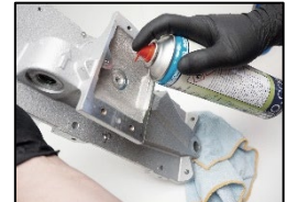
4. Clean the base plate for oil and dirt.
