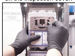
5. And right side until no dirt shown on the cotton sticks.
