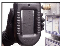
10. Install the u-tube manometer.
