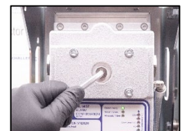
28. Remove the quick connection, and the oil mist detector is ready for operation!
