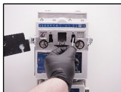
2. Clean the infrared sensor glasses on the right and left side with cotton sticks (Part no.: 10036) and technical alcohol (Part no.: 10035).
