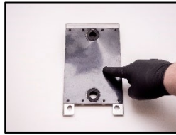
2. Check the measuring head gasket (Part no.: 10969). If damaged, replace the gasket.
