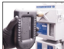
3. Install the u-tube manometer.
