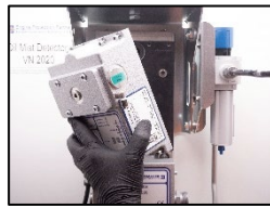
2. Disconnect the measuring head from the base plate.
