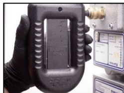
6. Connect the u-tube manometer and adjust the negative pressure to 60.00 mmWC!
