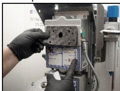
21. Replace the inspection seal.
