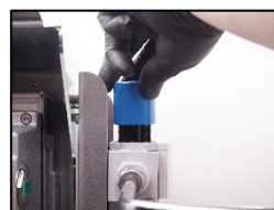
11. Adjust the air pressure to 60.00 mmWC!
