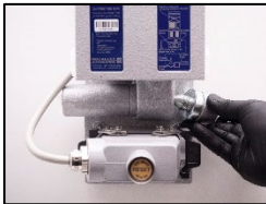
1. Disconnect the ejector input.
