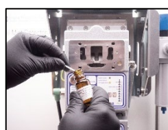
3. Use the cleaning fluid and cotton sticks.
