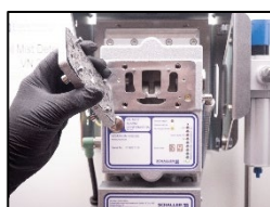
2. Open the inspection cover.
