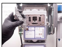
2. Open the inspection cover.
