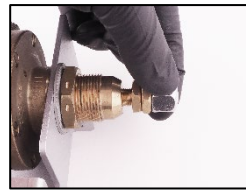
11. Adjust the air pressure to 60.00 mmWC!
