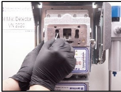
5. And clean the diode until the glass is clean.
