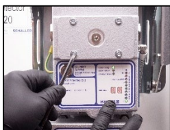
25. Install the inspection cover.
