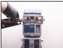
1. Open the inspection cover.
