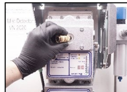
7. Install the quick connection.
