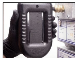
27. Connect the u-tube manometer and adjust the negative pressure to 60.00mmWC!
