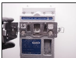
1. Open the inspection cover.
