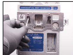
3. Clean the glasses with a cotton stick (Part no.: 10036) and technical alcohol (Part no.: 10035).
