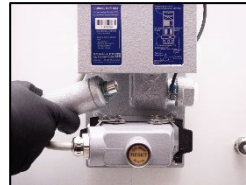
3. Reinstall the ejector output.
