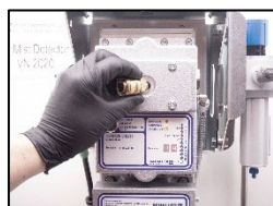
5. Connect the quick connection.
