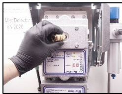
1. Install the quick connection.
