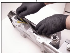
9. Install the pipe connection box.
