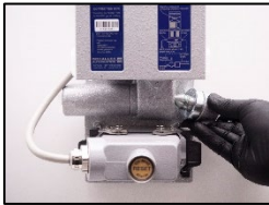
1. Disconnect the ejector input.
