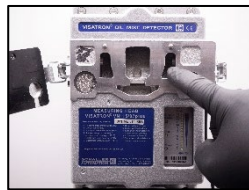
2. The infrared filter glasses may be dirty.
