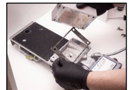
8. Replace the valve box gasket.
