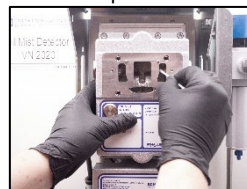
23. Clean the infrared sensor glass on the right side.
