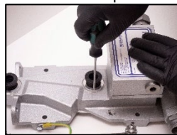
10. Disconnect the lower flexible bellow.
