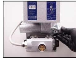
3. Reinstall the ejector input.
