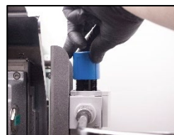
3. Adjust the air pressure to 60.00 mmWC!
