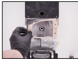
6. Change the valve box seal (Part nr.: 10405).
