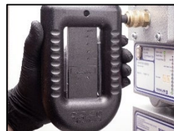
27. Connect the u-tube manometer and adjust the negative pressure to 60.00mmWC!
