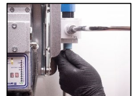
4. Unscrew the black plastic disc and remove the dirty filter.
