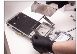
8. Replace the valve box gasket.
