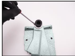
10. Replace the flexible bellows, included the mounting system kit (Part nr.: 10991).
