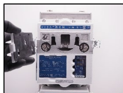
13. Open the inspection cover.
