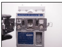
1. Open the inspection cover.
