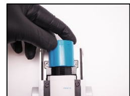
4. Turn up the pressure until it reaches 60 mmWC!
