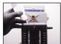
8. Fill in slacked water in the u-tube manometer.
