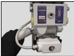
1. Disconnect the ejector input.
