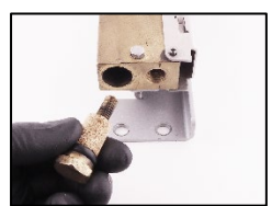
5. Insert the new gasket and filter onto the plug as shown.
