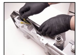
16. Reinstall the vibration damping plate.
