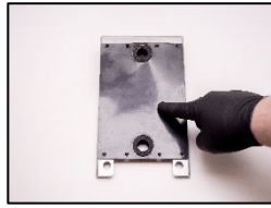
2. Check the measuring head gasket (Part no.: 10022). If damaged, replace it.
