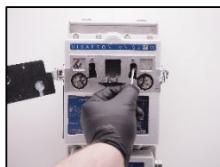
2. Clean the infrared sensor glasses on the right and left side with cotton sticks (Part no.: 10036) and technical alcohol (Part no.: 10035).
