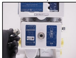
21. Change the screw plug seal \frac{1}{2} " (Part nr.: 10209).
