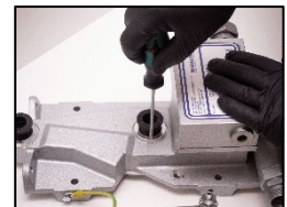
12. Unscrew the 2 pc. screws and remove the fastening ring for the lower bellow.
