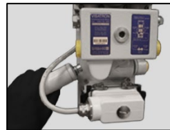
3. Reinstall the ejector input.
