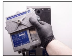
3. If voltage is ok – remove the measuring head.
