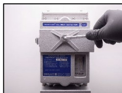
2. Remove the plug at the inspection cover.
