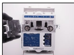
13. open the inspection cover
