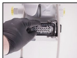
23. Check all leaders in the main socket. If bad condition – replace! (Part nr.: 10905)
