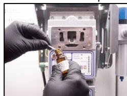
22. Use the cleaning liquid and cotton sticks
