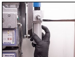
2. Hold the filter cage one hand and pull the blue tab down with your thumb.
