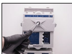
18. change the screw plug seal 1/4" for inspection cover (Part nr.: 10082)
