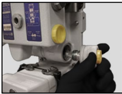
1. Disconnect the ejector input
