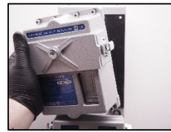
3. dismount the measuring head
