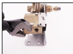
6. Insert the plug and tighten.
