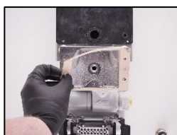
6. Change the valve box seal (Part nr.: 10405)
