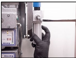
1. Replace the pressure regulator.
