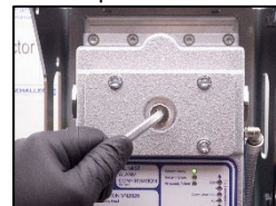
7. Remove the quick connection, and the oil mist detector is ready for operation!
