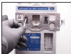
17. clean the infrared sensor glasses with cotton sticks and alcohol (Part nr.: 10036 & 10035)
