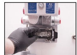
24. Check all leaders in the main socket. If bad condition – replace! (Part nr.: 10033)
