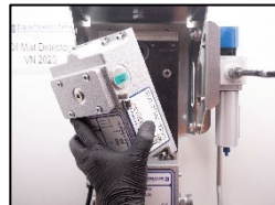
2. Remove the measuring head
