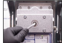
8. Install the plug and the detector is ready for operation!
