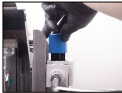
5. Adjust the air pressure to 60.00 mmWC.
