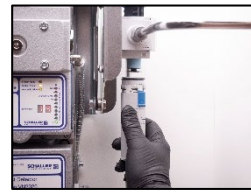
3. Turn the filter housing to the left and pull the housing down
