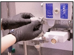
2. Remove the pipe from oil mist detector.
