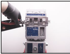
1. Open the inspection cover
