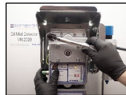
3. Replace the measuring head. Tighten the captive screws crosswise with torque of 4.5Nm
