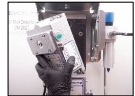
8. Install the measuring head
