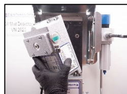
2. Remove the measuring head
