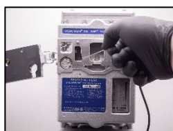
2. Use cleaning needle (Part no.: 10135) and clean the fresh air bores on the left and right side
