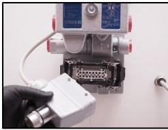
1. Remove the RESET task house
