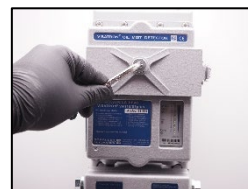
19. change the screw plug seal 1/4" for inspection cover (Part nr.: 10082)
