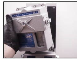
3. dismount the measuring head
