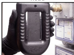
13. The negative pressure into the measuring head should be 60.00 mmWC. Adjust if necessary!
