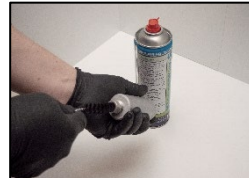
7. Clean the ejector in and out nozzle free for oil and dirt.
