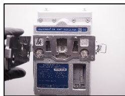
14. open the inspection cover
