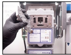
2. Open the inspection cover
