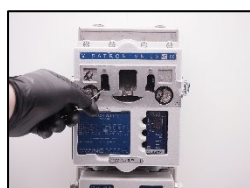
17. clean the bores with cleaning needle (Part nr.: 10135)
