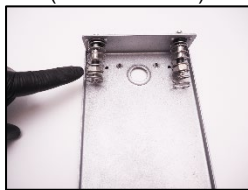
9. change the upper and lower elastic mounting system (Part nr.: 10018 & 10019)
