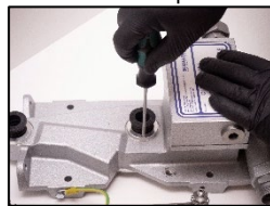
10. Disconnect the lower flexible bellow
