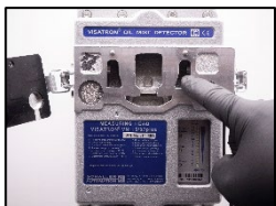
2. The infrared filter glasses may be dirty
