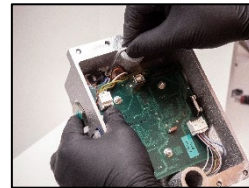
7. Position the securing clamp over the battery. Tighten the screw connection to 2.5 Nm
