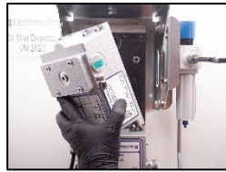
2. Remove the measuring head
