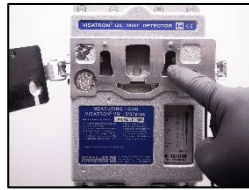
2. The infrared filter glasses may be dirty
