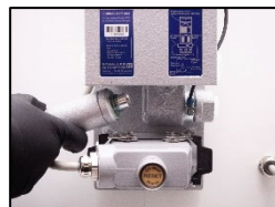
3. Reinstall the ejector output.
