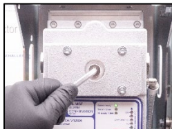
9. Open the plug at the cover on the measuring head
