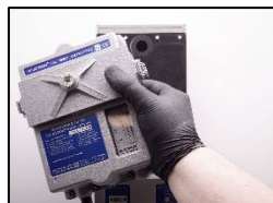
1. Replace the measuring head with an exchange unit.
