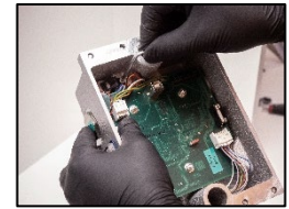
4. Loosen the screw of the security clamp, turn the security clamp to the side
