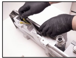
14. Replace the suspensions if necessary! Install the flexible damping plate back on the base plate
