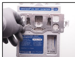
18. clean the bores with cleaning needle (Part nr.: 10135)
