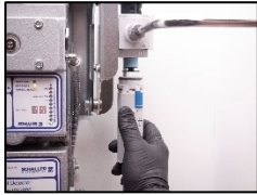
5. Re-install the housing
