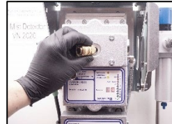
7. Install the quick connection.
