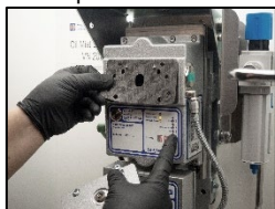
21. Replace the inspection seal
