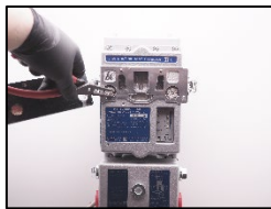
1. Open the inspection cover
