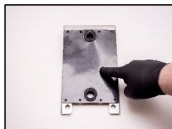
2. Check the measuring head gasket (Part no.: 10022). If damaged, replace it.
