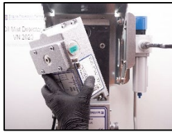
1. Disconnect the measuring head from the base plate.
