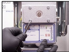
5. The negative pressure into the measuring head should be 60.00 mmWC. Adjust if necessary!
