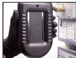
6. Connect the u-tube manometer and adjust the negative pressure to 60.00 mmWC
