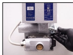
3. Reinstall the ejector input.
