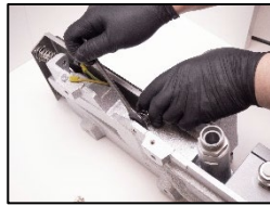
2. Remove the base plate from protection cover base.
