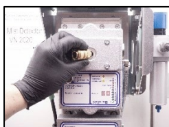
5. Connect the quick connection
