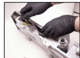
16. Reinstall the vibration damping plate.
