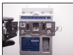
1. Open the inspection cover
