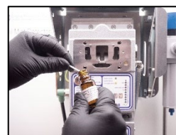
3. Use the cleaning fluid and cotton sticks.
