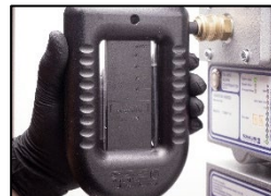
7. And adjust the pressure to 60.00 mmWC
