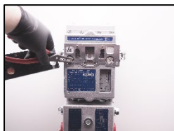
1. Open the inspection cover
