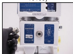
21. change the screw plug seal 1/2" (Part nr.: 10209)
