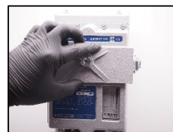
23. check the heating element if it is hot. If cold – replace!
