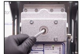
8. Open the inspection cover.
