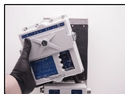
3. Install the new exchange measuring head. When starting up the OMD device, please check the negative pressure and adjust if necessary!
