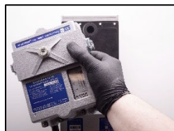
1. Remove the measuring head
