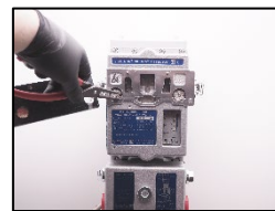
15. change the scavenging air filter (Part nr.: 10042)
