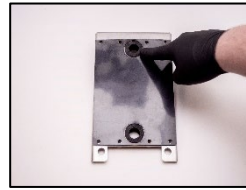
3. Check the flexible bellows (Part no.: 10023). If damaged, replace the flexible bellows
