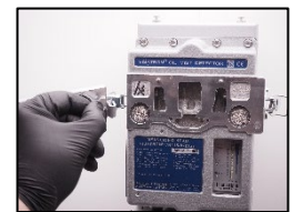
16. Change the seal for inspection cover (Part nr.: 10010/10166)
