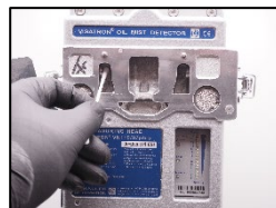
3. Clean the glasses with a cotton stick (Part no.: 10036) and technical alcohol (Part no.: 10035)
