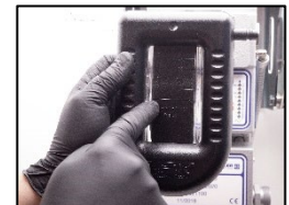
12. Fill up to marked line on the u-tube manometer
