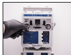
3. Clean the fresh air bores on the right and left side with a cleaning needle (Part no.: 10135)
