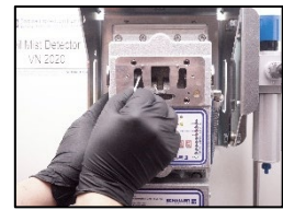
4. To clean the infrared sensor on left side
