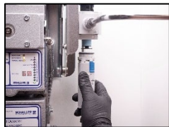
5. Re-install the housing
