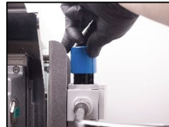
11. Adjust the air pressure to 60.00 mmWC.
