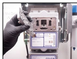
2. Open the inspection cover.
