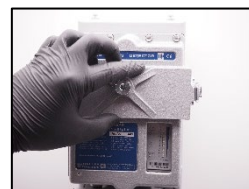
23. check the heating element if it is hot. If cold – replace!
