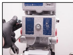
22. change the screw plug seal 1/2" (Part nr.: 10209)
