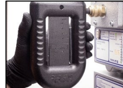
7. And adjust the pressure to 60.00 mmWC
