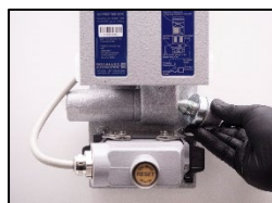
1. Disconnect the ejector input
