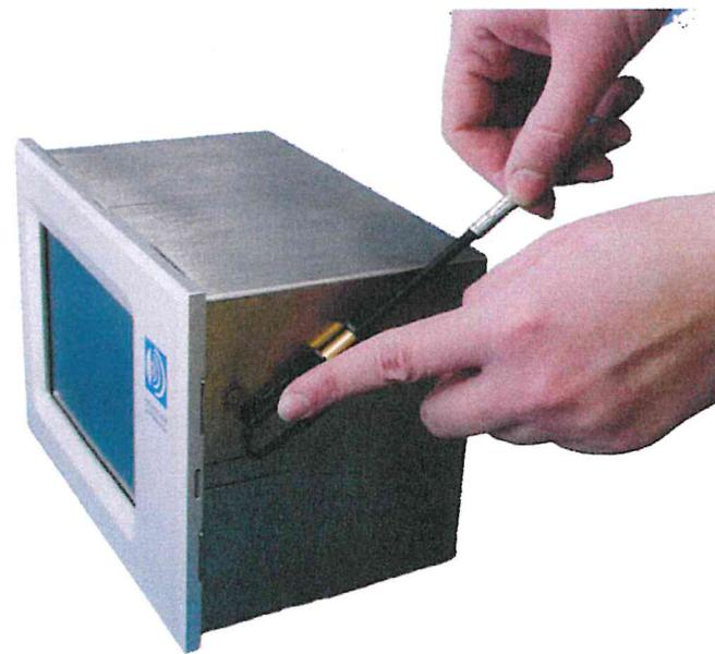
Figure 30: Mounting the fixing screws
