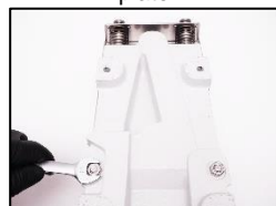
11. Install the new vibration plate to the base plate
