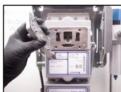
2. Open the inspection cover.
