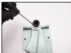
10. Replace the flexible bellows, included the mounting system kit (Part no.: 10991)
