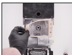
6. Change the valve box seal (Part no.: 10405)
