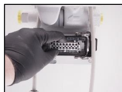
23. Check all leaders in the main socket. If bad condition – replace! (Part no.: 10905)
