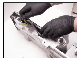
16. Reinstall the vibration damping plate.
