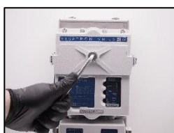
18. change the screw plug seal 1/4" for inspection cover (Part no.: 10082)
