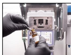
3. Use the cleaning fluid and cotton sticks.
