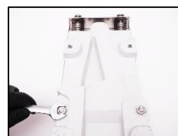
8. unscrew the vibration plate
