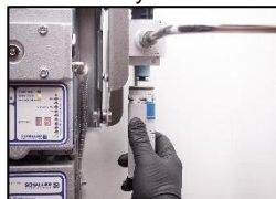
6. Reinstall the filter cage.
