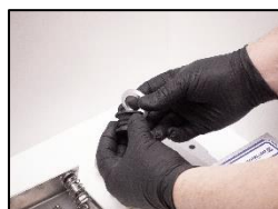
13. Check the lower bellow damage, replace if necessary.
