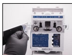
15. Change the seal for inspection cover (Part no.: 11180)
