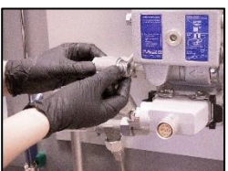
2. Remove the pipe from oil mist detector.
