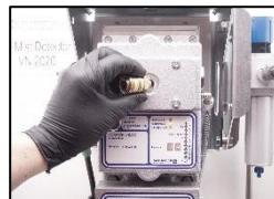
7. Install the quick connection.
