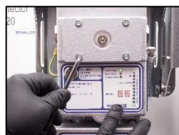
1. Remove the plug in the inspection cover.
