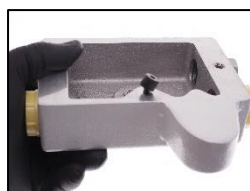
5. Change the small seal (Part no.: 10206)
