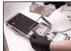
8. Replace the valve box gasket.
