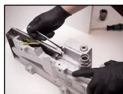
3. Unscrew the 4 pc. mounting bolts on the pipe connection box.
