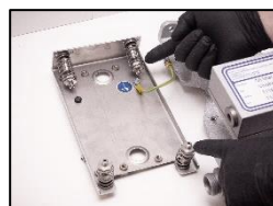
15. Check the upper and lower suspensions for any damage, replace if necessary.
