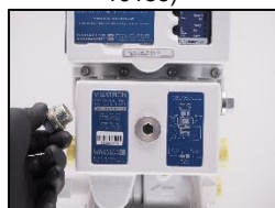
21. change the screw plug seal 1/2" (Part no.: 10209)
