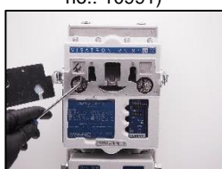
14. change the scavenging air filter (Part no.: 10042)
