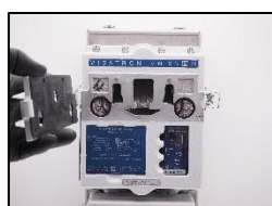
13. open the inspection cover
