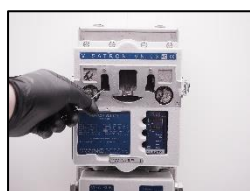
17. clean the bores with cleaning needle (Part no.: 10135)
