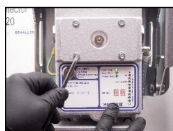
1. Loosen the captive screws on the inspection cover.
