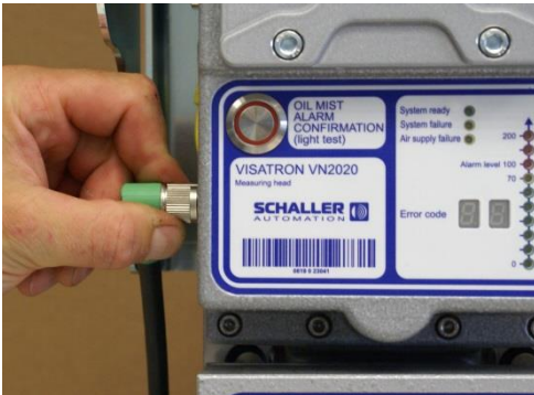
Figure 101: mounting of plug-in connector
