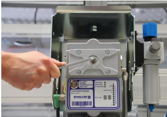
Figure 180: Inspection cover with screw plug
