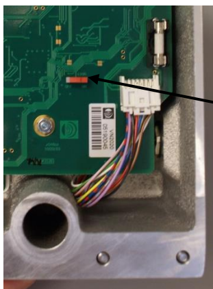
Figure 52: Switchable termination resistor
