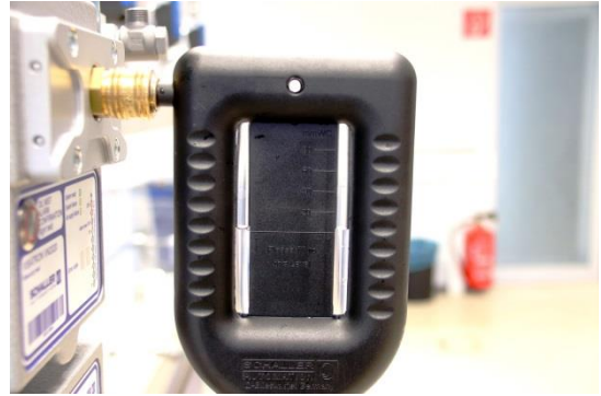
Figure 59: Negative pressure display on the U-tube manometer
