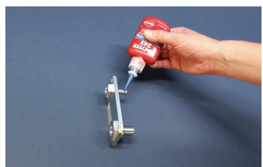
Figure 24: Screws with Loctite
