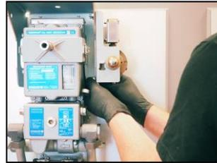
3. loosen the mounting screws on the old pressure regulator...
