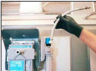
9. install the new flexible pipe to the existing air pipe on the engine. When this procedure is done-adjust the negative pressure to 60.00 mmWC. Turn on the power to the system, and make a system test with test plate kit no. 11072. After the test is done-the oil mist detector are ready for operation.
