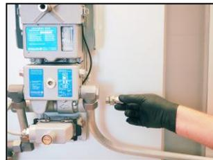
7. install the new connection plug on the ejector input...
