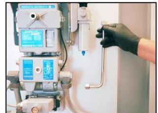
8. install the new steel main pipe between the ejector input the pressure regulator...
