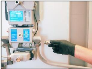
5. remove the old connection plug from the ejector input on the base plate...
