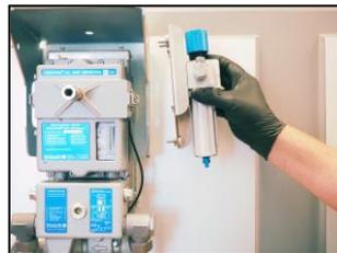
6. install the new pressure regulator, use the same holes into the protection cover...
