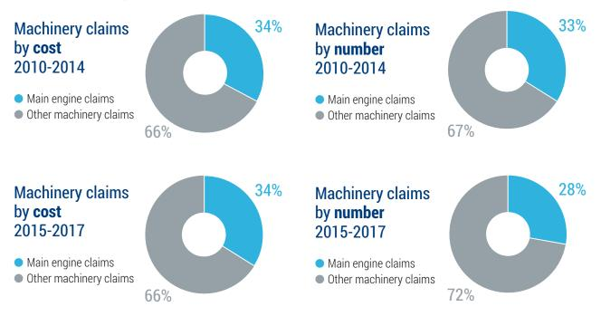
The trend in main damage claims in 2015 - 2017 is virtually unchanged, compared with 2010-2014, with main engine damage contributing to approximately a third of all machinery claims both in terms of cost and number of claims. The number of claims has reduced slightly during the period 2015 - 2017, but overall claims costs have remained the same.
