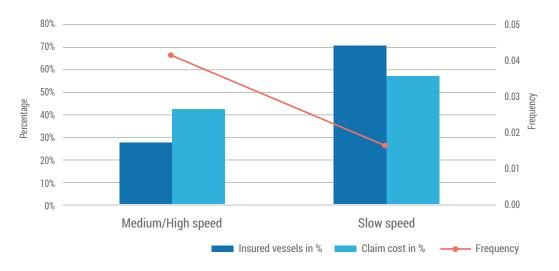
Medium/high speed engines are 2.5 times more frequently damaged compared with slow speed engines. They also have a disproportionate claims cost (43%) in relation to the number of insured vessels (28%).
