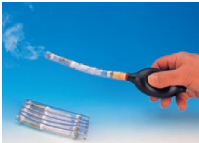
Figure 28: VISATRON® VN301 plus /VN301 plus EX Mist Generator. Tubule consisting of ethylenediamine and acetic acid for mist generation, hand pump.
