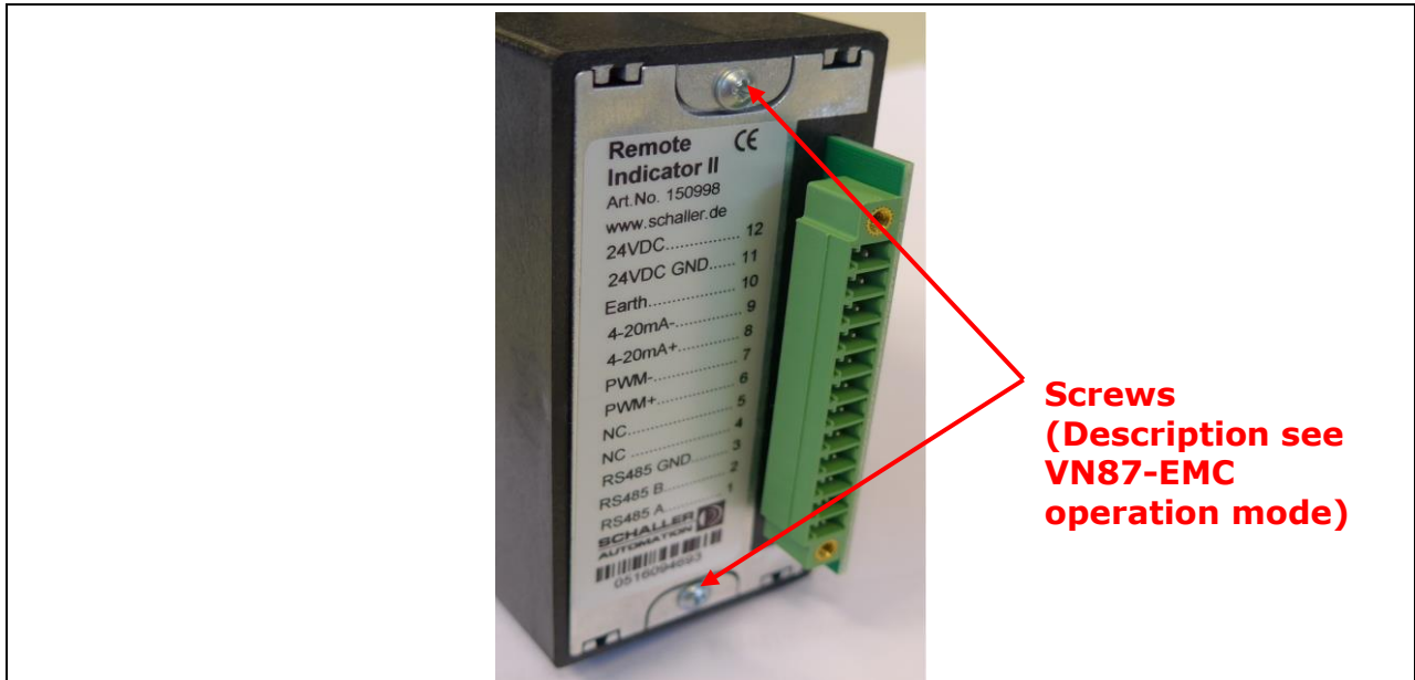
Figure 07: Connector at the rear side of the Remote Indicator II
