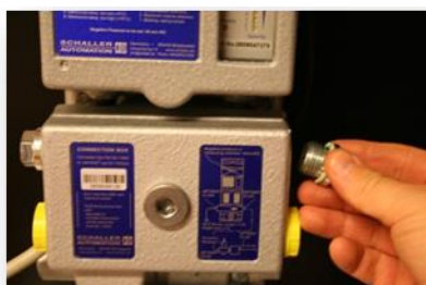
change the screw plug seal 1/2" (P/n.: 10209)... check the heating element if it is hot- if cold socket... replace (P/n.: 10033)
