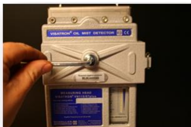
change the screw plug seal 1/4" for inspection cover... close the inspection cover... (P/n.: 10082)
