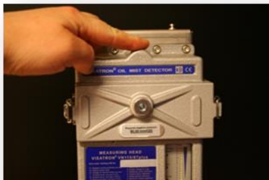
change the screw plug seal 1/2" (P/n.: 10209)... check the heating element if it is hot- if cold socket... replace (P/n.: 10033)
