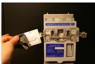
change the seal for inspection cover... clean the infra- red sensor glasses with cotton sticks and alcohol...clean the bores with cleaning needle (P/n.: 10010/ 10166)
