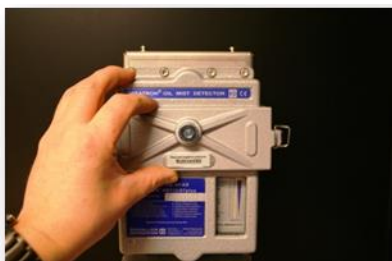
change the screw plug seal 1/4" for inspection cover... close the inspection cover... (P/n.: 10082)
