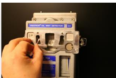
change the seal for inspection cover... clean the infra- red sensor glasses with cotton sticks and alcohol...clean the bores with cleaning needle (P/n.: 10010/ 10166)
