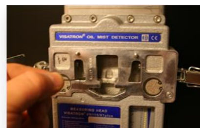
change the seal for inspection cover... clean the infra- red sensor glasses with cotton sticks and alcohol...clean the bores with cleaning needle (P/n.: 10010/ 10166)
