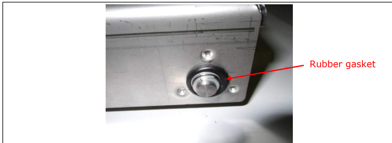
Figure 41: Step 2 is to press out the 4 rubber gaskets with a blunt tool and finally to remove the carrier plate
