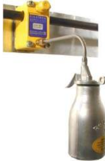
Figure 27: Filling pump inserted and fixed in the siphon block
