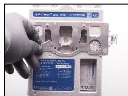
18. Clean the bores with cleaning needle.
