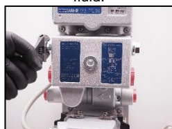
21. Unscrew the plugs at the connection case.
