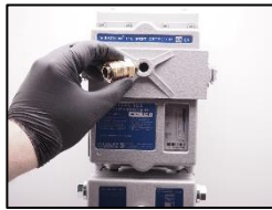
1. Install the quick connection.
