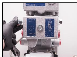
22. Change the screw plug seal 1/2\"/>
