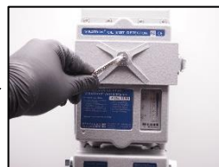
19. Change the screw plug seal 1/4\"/>
