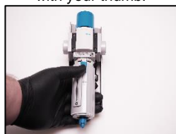
6. Reinstall the filter cage.
