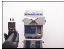
2. Connect the u-tube manometer.
