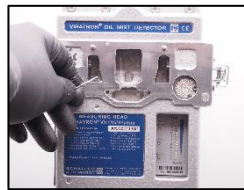
3. Clean the fresh air bones in the measuring head. Use the cleaning needle.
