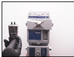
1. Check the negative pressure with a u-tube manometer. Adjust if necessary! Setting level is 55.00 – 65.00 mmWC!
