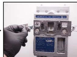
16. Change the seal for inspection cover.
