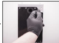
12. Change the measuring head seal.
