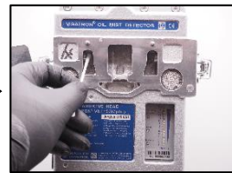
4. Clean the infrared sensor glasses at the left and the right side inside the measuring head. Use cotton sticks and cleaning fluid.
