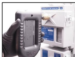
10. Install the u-tube manometer.
