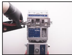
2. Replace the sintered bronze air filter/fresh air filter.
