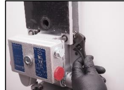
8. Unscrew the vibration plate.
