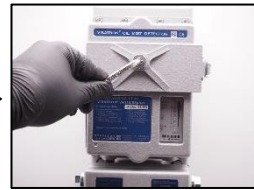
4. Install the inspection cover plug.
