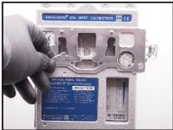
3. Clean the fresh air bones in the measuring head. Use the cleaning needle.
