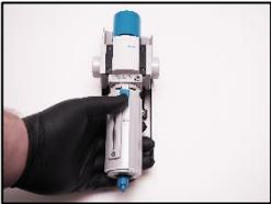
6. Reinstall the filter cage.
