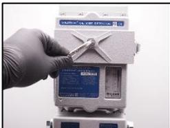
19. Change the screw plug seal 1/4" for inspection cover.
