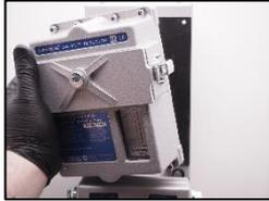
3. Install the new exchange measuring head. When starting up the OMD device, please check the negative pressure and adjust if necessary! See procedure 1. Make final test of the system to ensure that oil mist detector operation is safe.
