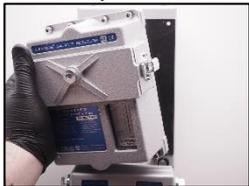
13. Reinstall the measuring head to the vibration plate.
