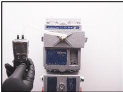
1. Check the negative pressure with a u-tube manometer. Adjust if necessary! Setting level is 60,00 mmWC!
