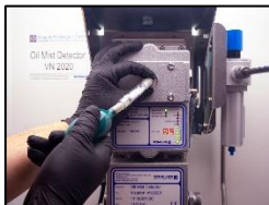
5. Pump smoke until the oil mist alarm is realised.
