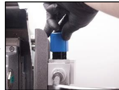
11. Adjust the air pressure to 55.00 - 65.00 mmWC!
