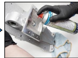
4. Clean the base plate for oil and dirt.
