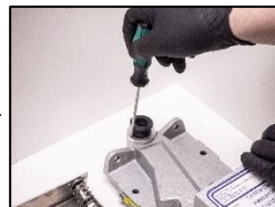
10. Unscrew the 2 pc. screws, and remove the fastening ring for the upper bellow.
