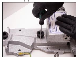
14. Reinstall the fastening ring and ensure correct position of the bellows.
