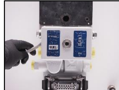
7. Reconnect the connection case to the base plate.
