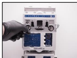
17. Clean the bores with cleaning needle.
