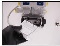
2. Disconnect the RESET connector.
