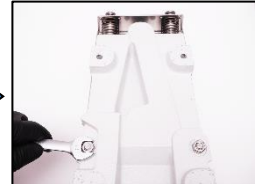
8. Unscrew the vibration plate.
