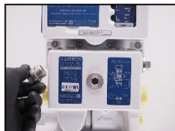
21. Change the screw plug seal 1/2".
