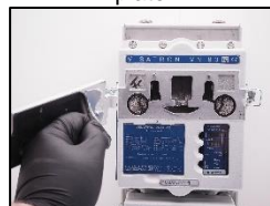
15. Change the seal for inspection cover.
