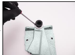
10. Replace the flexible bellows.
