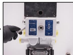
4. Disconnect the connection case.
