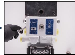
4. Disconnect the connection case.
