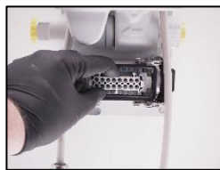
21. Check all leaders in the main socket. If bad condition – replace!
