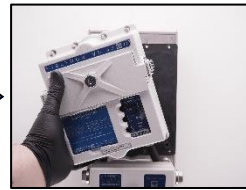
3. Dismount the measuring head.
