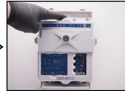
20. Check the heating element if it is hot. If cold – replace!
