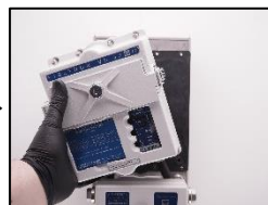
3. Dismount the measuring head.
