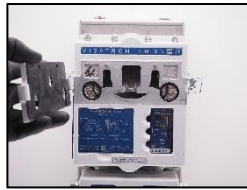
13. Open the inspection cover.
