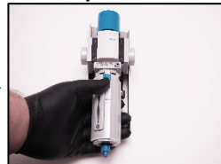
6. Reinstall the filter cage.
