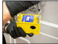
11. Tighten the screws until the siphon block holds together.
