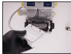
2. Disconnect the RESET task connector.
