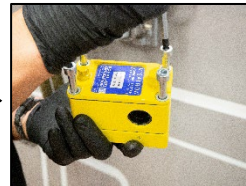
7. Unscrew the screws completely
