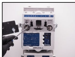
2. Replace the fresh air restrictor and the scavenging air filter.
