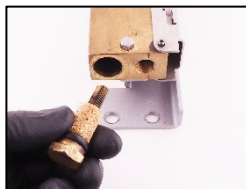
5. Screw in the filter plug with new parts on it.
