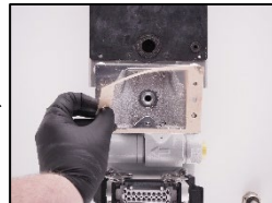
6. Change the valve box seal.
