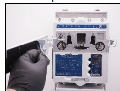
15. Change the seal for inspection cover.
