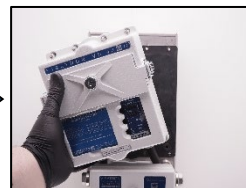
3. Dismount the measuring head.
