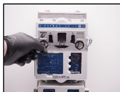
17. Clean the bores with cleaning needle.
