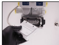
2. Disconnect the RESET task connector.
