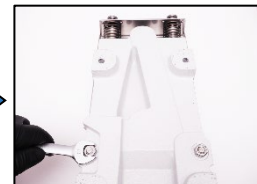
8. Unscrew the vibration plate and check for damage.
