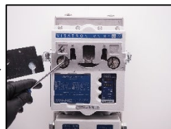
14. Change the scavenging air filter.
