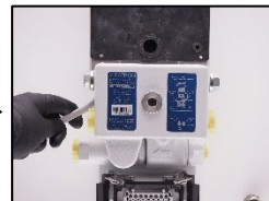
7. Reconnect the connection case to the baseplate.
