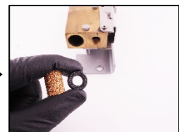
4. Replace both the o-ring and filter.
