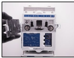
1. Open the inspection cover.
