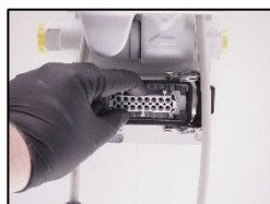
21. Check all leaders in the main socket. If bad condition – replace!
