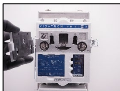
1. Open the inspection cover.
