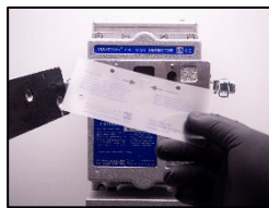
2. The oil mist detector needs to be in operation mode with negative pressure set to 60mmWC.
