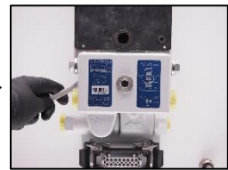
4. Disconnect the connection case.
