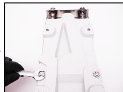
10. Install the vibration plate to the baseplate.
