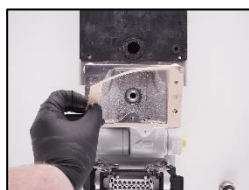
6. Change the valve box seal.
