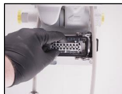
15. Check all leaders in the main socket. If bad conditions – replace the connection socket!
