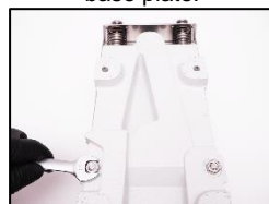
11. Install the new vibration plate to the base plate.
