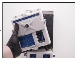
3. Dismount the measuring head.
