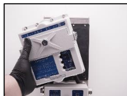
14. Replace the measuring head.
