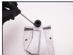
10. Change the flexible bellows.
