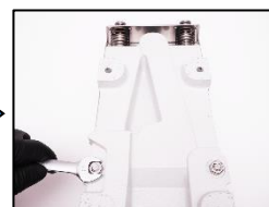
8. Unscrew the vibration plate.
