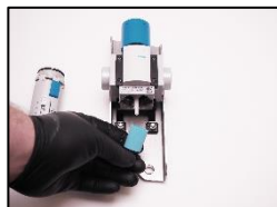
5. Screw in the new filter counter clockwise and make sure that it is aligned for installation.
