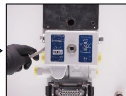
4. Disconnect the connection case.
