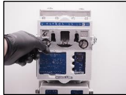
17. Clean the bores with cleaning needle.
