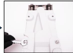
8. Unscrew the vibration plate and check for damage.
