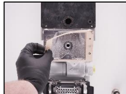
6. Change the valve box seal.
