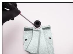
10. Replace the flexible bellows.
