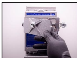
1. Open the inspection cover on the measuring head.
