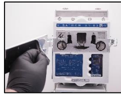
15. Change the seal for inspection cover.
