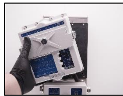
3. Dismount the measuring head.
