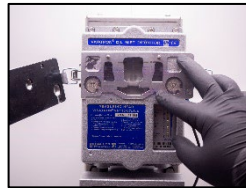
3. Place the test plate over the open chamber – the test plate will be sucked into position by the vacuum in the measuring head.
