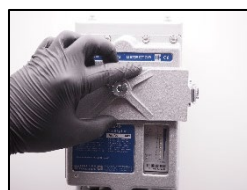
3. Close the inspection cover.
