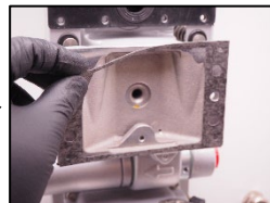
6. Check the valve box seal.
