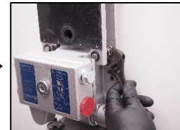
8. Unscrew the vibration plate.
