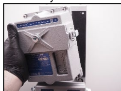
13. Reinstall the measuring head at the vibration plate.
