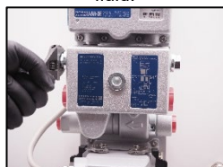
21. Unscrew the plugs at the connection case.
