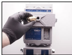
1. Turn off the air and install the quick connection.
