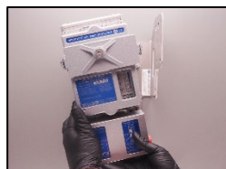
2. Disconnect the used oil mist detector.
