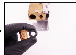
4. Replace both the o-ring and filter.
