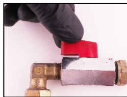
1. Stop the engine and close the incoming air pressure.
