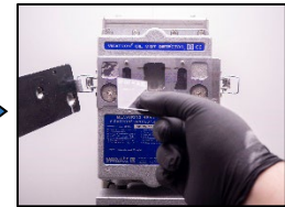
4. Press the 10% glass into the slit in the test plate. Ensure the glass is in a straight vertical position.
