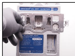
18. Clean the bores with cleaning needle.
