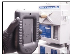
3. Insert it into the quick connection and adjust the pressure to 60mmWC.
