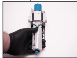
6. Reinstall the filter cage.
