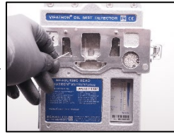
3. Clean the bores with cleaning needle.
