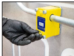
17. Unscrew the pump and reinstall the screw.
