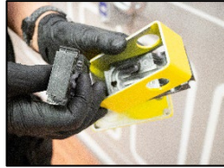
9. Remove and check the rubber inserts.
