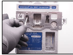
2. Clean the infrared sensor glasses with cotton sticks and cleaning fluid.
