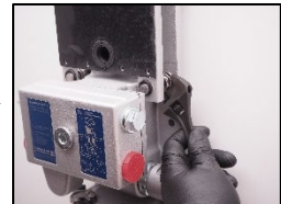
8. Unscrew the vibration plate.
