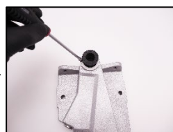
10. Check the flexible bellows for any damage.
