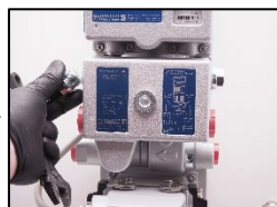
22. Change the screw plug seal 1/2".
