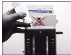
2. Fill in slacked water in the u-tube manometer to the middle line.
