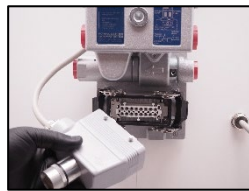
2. Disconnect the RESET task connector.
