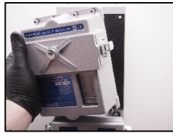
13. Reinstall the measuring head at the vibration plate.
