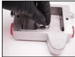
5. Check the small seal.
