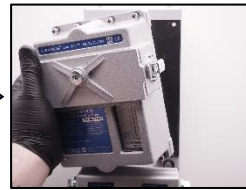
3. Dismount the measuring head.
