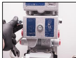
22. Change the screw plug seal 1/2".
