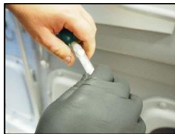
1. With the crank cases open, break glass capsules in the smoke test tube to activate smoke production.
