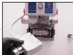
2. Disconnect the RESET task connector.
