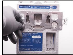
18. Clean the bores with cleaning needle.
