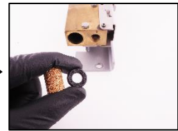
4. Replace both the o-ring and filter.
