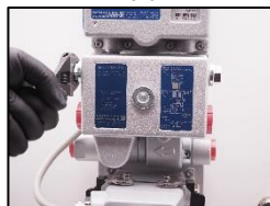
21. Unscrew the plugs at the connection case.
