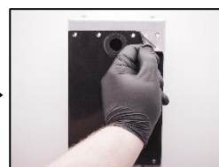
12. Change the measuring head seal.
