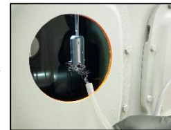
2. Place the test tube right under sampling funnel and pump smoke into it until the measuring head enters alarm mode.
