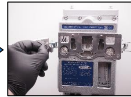
16. Change the seal for inspection cover.
