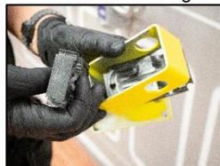
9. Remove and check the rubber inserts.
