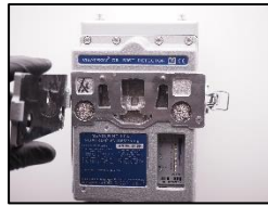
14. Open the inspection cover.
