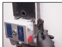
8. Unscrew the vibration plate.
