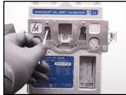
17. Clean the infrared sensor glasses with cotton sticks and cleaning fluid.
