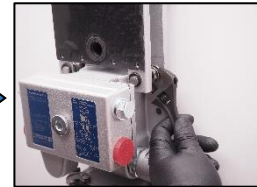
8. Unscrew the vibration plate...
