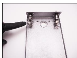
9. Change the upper and lower elastic mounting system.
