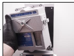
3. Dismount the measuring head.
