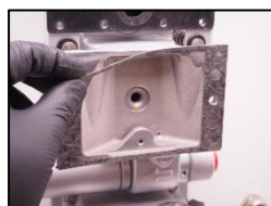
6. Change the valve box seal.
