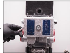
7. Reconnect the connection case to the baseplate.
