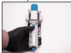
6. Reinstall the filter cage.
