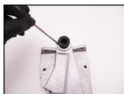
10. Change the flexible bellows.
