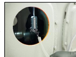
2. Place the test tube right under sampling funnel and pump smoke into it until the measuring head enters alarm mode.
