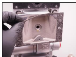
6. Change the valve box seal.
