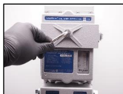
19. Change the screw plug seal 1/4\"/>
