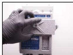
14. Check the heating element if it is hot. If cold – replace!
