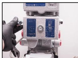
22. Change the screw plug seal 1/2\"/>
