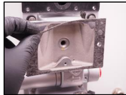
6. Change the valve box seal.
