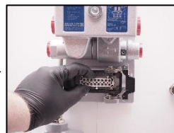
15. Check all leaders in the main socket. If bad condition – replace!
