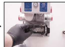
24. Check all leaders in the main socket. If bad condition - replace!
