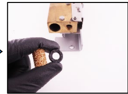
4. Replace both the o-ring and filter.
