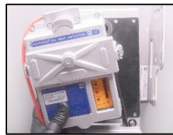
3. Dismount the measuring head.
