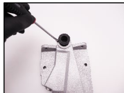
10. Change the flexible bellows.
