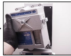
3. Dismount the measuring head.
