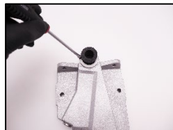
10. Change the flexible bellows.
