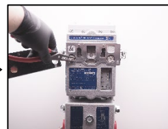
15. Change the scavenging air filter.
