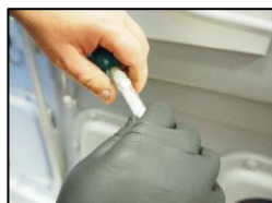
1. With the crank cases open, break glass capsules in the smoke test tube to activate smoke production.
