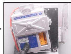
3. Dismount the measuring head.
