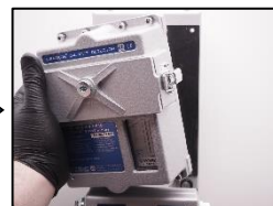
3. Dismount the measuring head.
