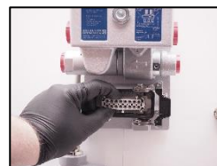
24. Check all leaders in the main socket. If bad condition – replace!
