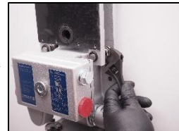
8. Unscrew the vibration plate.
