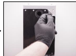
12. Change the measuring head seal.
