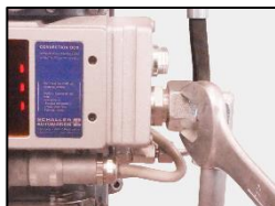
1. Loosen the pipe connections from the connection casing.
