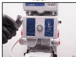
21. Unscrew the plugs at the connection case.
