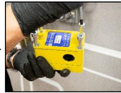
7. Unscrew the screws completely
