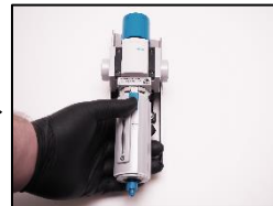
3. Turn the filter cage clockwise and pull out downwards.
