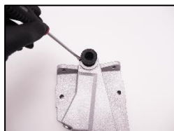
10. Change the flexible bellows.
