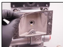
6. Change the valve box seal.
