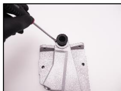
10. Change the flexible bellows.
