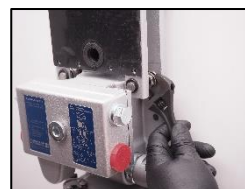
8. Unscrew the vibration plate.
