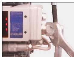
3. Tighten the pipe to the connection casing.
