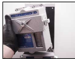
3. Dismount the measuring head.
