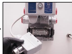
2. Disconnect the RESET task connector.
