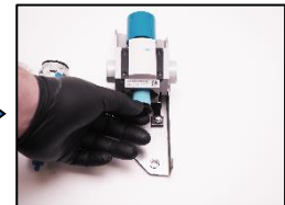
4. Unscrew the black plastic disc and remove the dirty filter.
