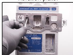
17. Clean the infrared sensor glasses with cotton sticks and cleaning fluid.
