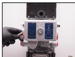
7. Reconnect the connection case to the base plate.
