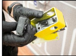
9. Remove and check the rubber inserts.
