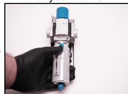
6. Reinstall the filter cage.
