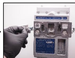
16. Change the seal for inspection cover.
