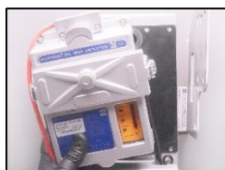
14. Replace the measuring head.
