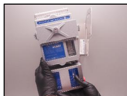
2. Disconnect the used oil mist detector.
