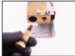
5. Screw in the filter plug with new parts on it.
