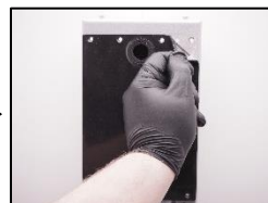
12. Change the measuring head seal.
