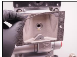
6. Change the valve box seal.
