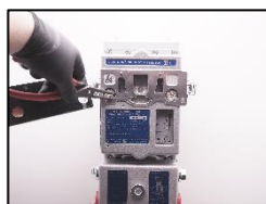
15. Change the scavenging air filter.
