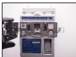
14. Open the inspection cover.
