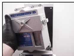
14. Replace the measuring head.
