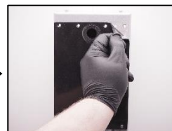
12. Change the measuring head seal.
