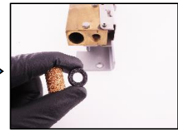
4. Replace both the o-ring and filter.
