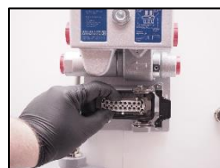
16. Check all leaders in the main socket. If bad conditions – replace the connection socket!
