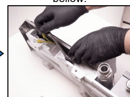
16. Reinstall the vibration damping plate.
