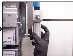
2. Hold the filter cage one hand and pull the blue tab down with your thumb.
