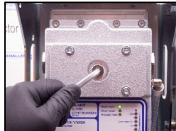
1. Remove the plug in the inspection cover.
