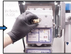
7. Install the quick connection.
