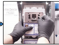
4. Clean the glass on the transmitter diode on the right side until it is clean.
