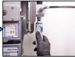
6. Reinstall the filter cage.
