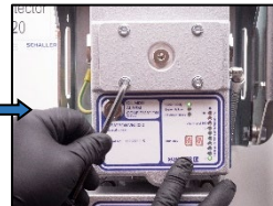
7. Close the inspection cover and hand tight the captive screws.
