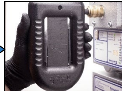
10. Install the u-tube manometer.
