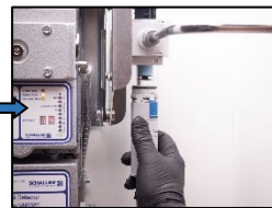
3. Turn the filter cage clockwise and pull out downwards.
