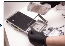
8. Replace the valve box gasket.
