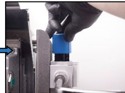
11. Adjust the air pressure to 55.00 – 65.00 mmWC!
