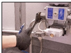
1. Loosen the main pipe connection.
