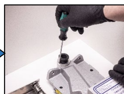
10. Unscrew the 2 pc. screws, and remove the fastening ring for the upper bellow.
