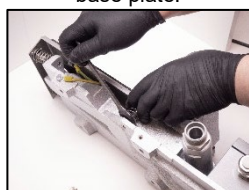
9. Install the pipe connection box.
