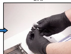
11. Check the upper bellow for damage, replace if necessary.
