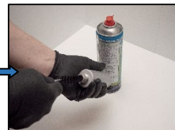
7. Clean the ejector in and out nozzle free for oil and dirt.
