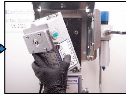
18. Install the measuring head and tighten the captive screws with a torque of 4,5 Nm.
