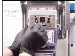
5. And clean the diode until the glass is clean.
