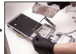
8. Replace the valve box gasket.
