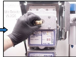
7. Install the quick connection.
