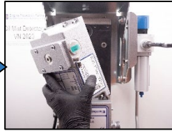
18. Install the measuring head and tighten the captive screws with a torque of 4,5 Nm.
