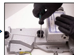
12. Unscrew the 2 pc. screws and remove the fastening ring for the lower bellow.
