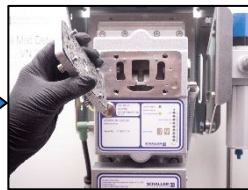
2. Open the inspection cover.
