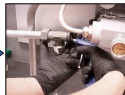
3. Blow compressed air into the main pipe for few seconds so collected oil will drain back to the engine.
