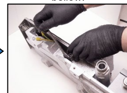
16. Reinstall the vibration damping plate.
