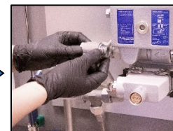
2. Remove the pipe from oil mist detector.
