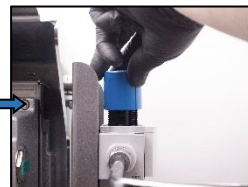
11. Adjust the air pressure to 55.00 – 65.00 mmWC!
