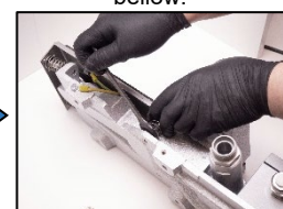
16. Reinstall the vibration damping plate.
