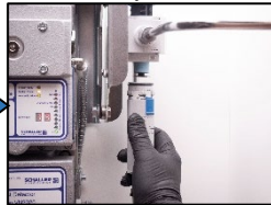
6. Reinstall the filter cage.
