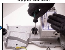
14. Reinstall the fastening ring and ensure correct position of the bellows.
