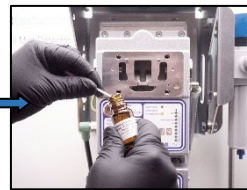
3. Use the cleaning fluid and cotton sticks.
