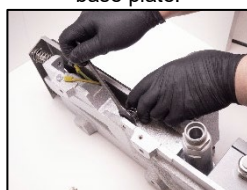
9. Install the pipe connection box.
