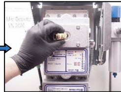
7. Install the quick connection.
