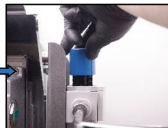
11. Adjust the air pressure to 55.00 – 65.00 mmWC!
