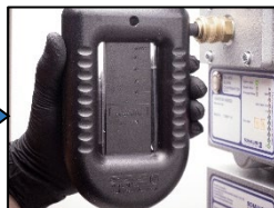
10. Install the u-tube manometer.
