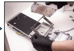
8. Replace the valve box gasket.
