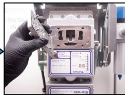
2. Open the inspection cover.
