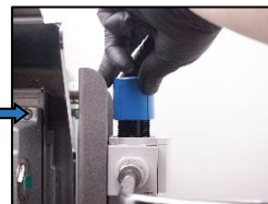
11. Adjust the air pressure to 55.00 – 65.00 mmWC!
