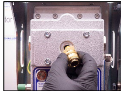
2. Install the test plug at the inspection cover.
