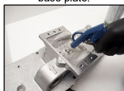
5. Use compressed air to the air channels into the base plate.
