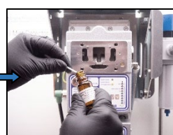
3. Use the cleaning fluid and cotton sticks.
