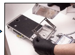
8. Replace the valve box gasket.
