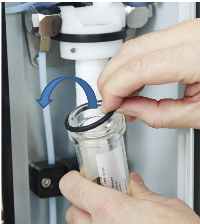
Figure 56 Replacing the sealing ring
