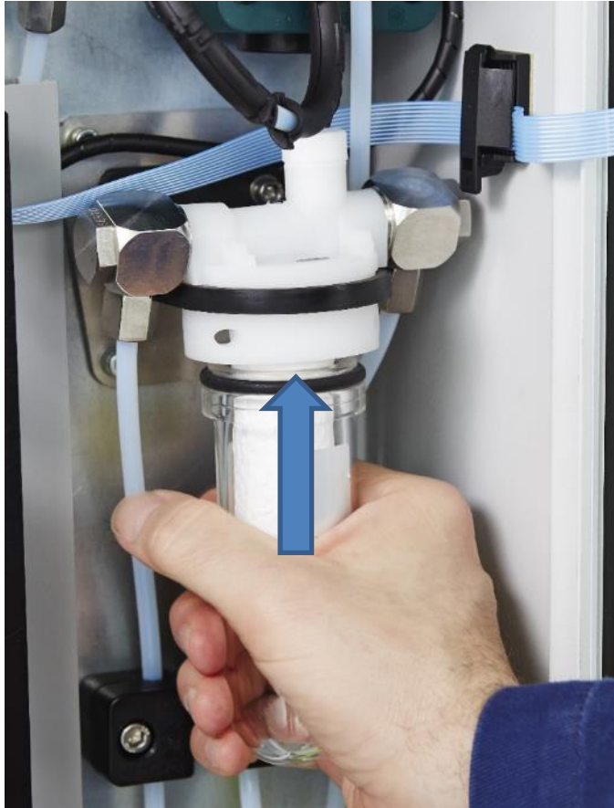
Figure 57 Pushing on the filter bowl
