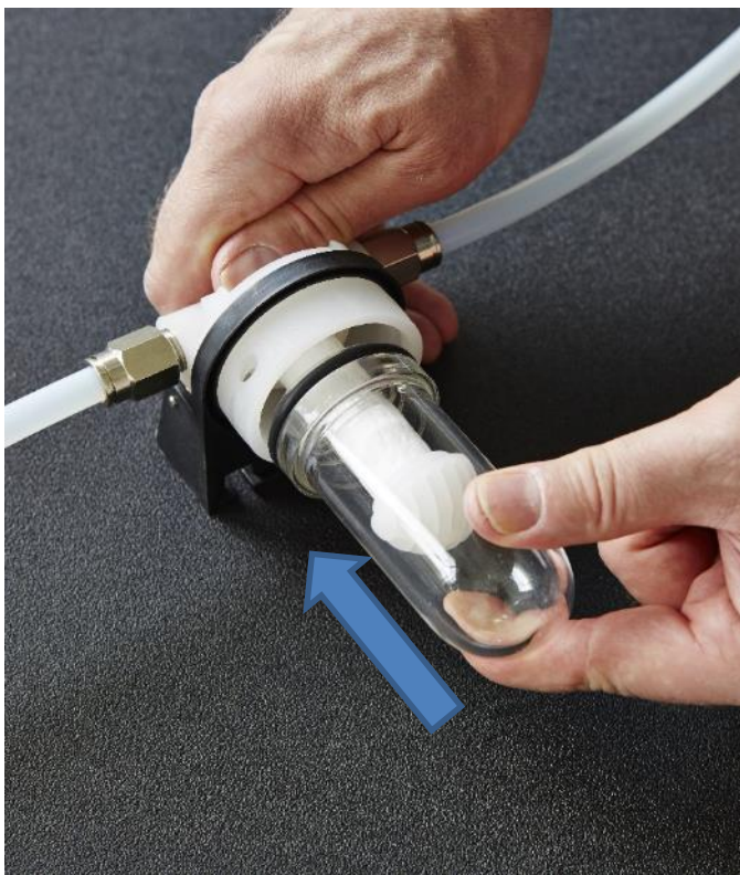
Figure 64 Pushing on the filter bowl on the coalescing filter
