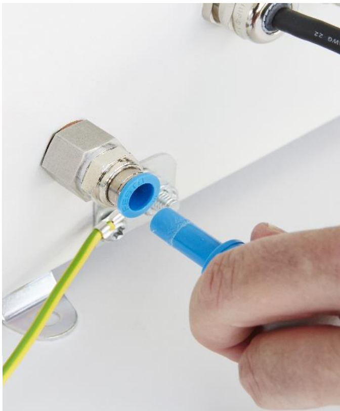
Figure 66 Replacing the filter element of the environmental air input
