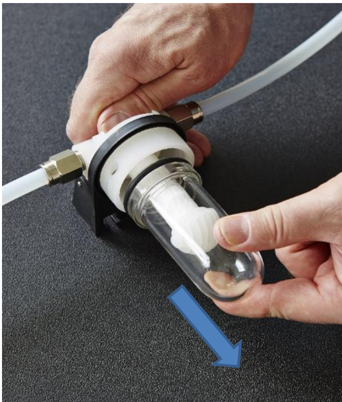
Figure 60 Removing the filter bowl on the coalescing filter
