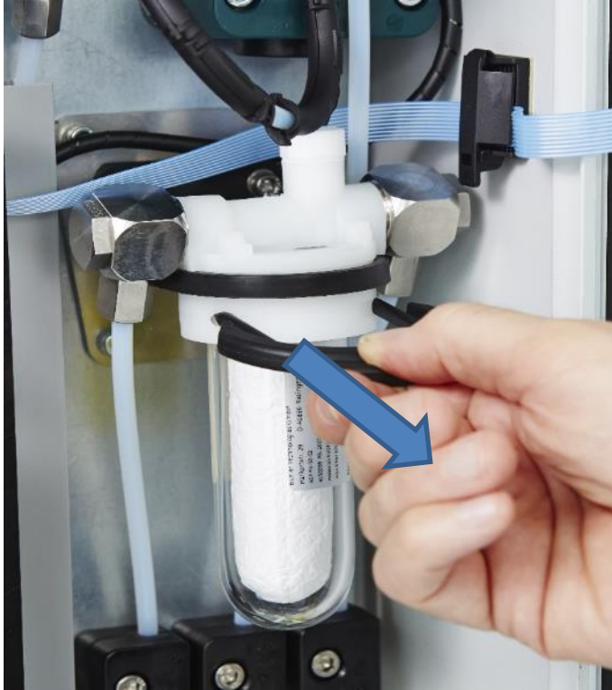
Figure 52 Releasing the filter bowl lock
