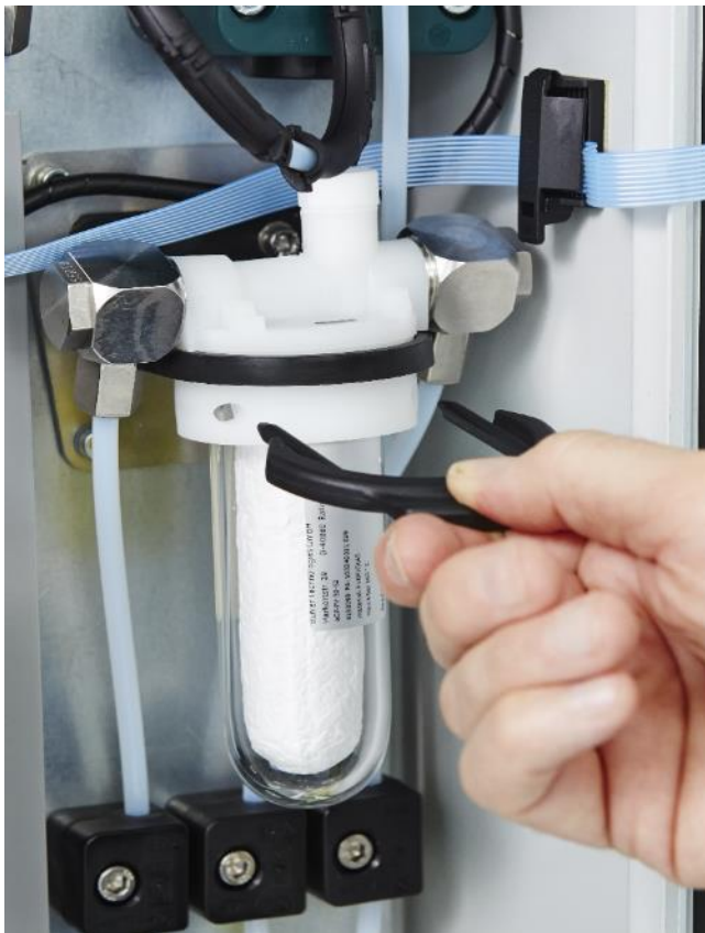
Figure 58 Inserting the filter bowl retaining bracket
