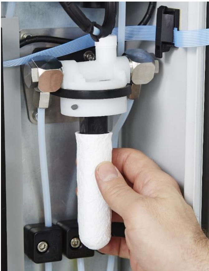
Figure 54 Replacing the filter element
