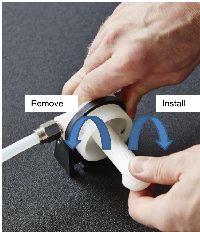
Figure 61 Removing the filter element
