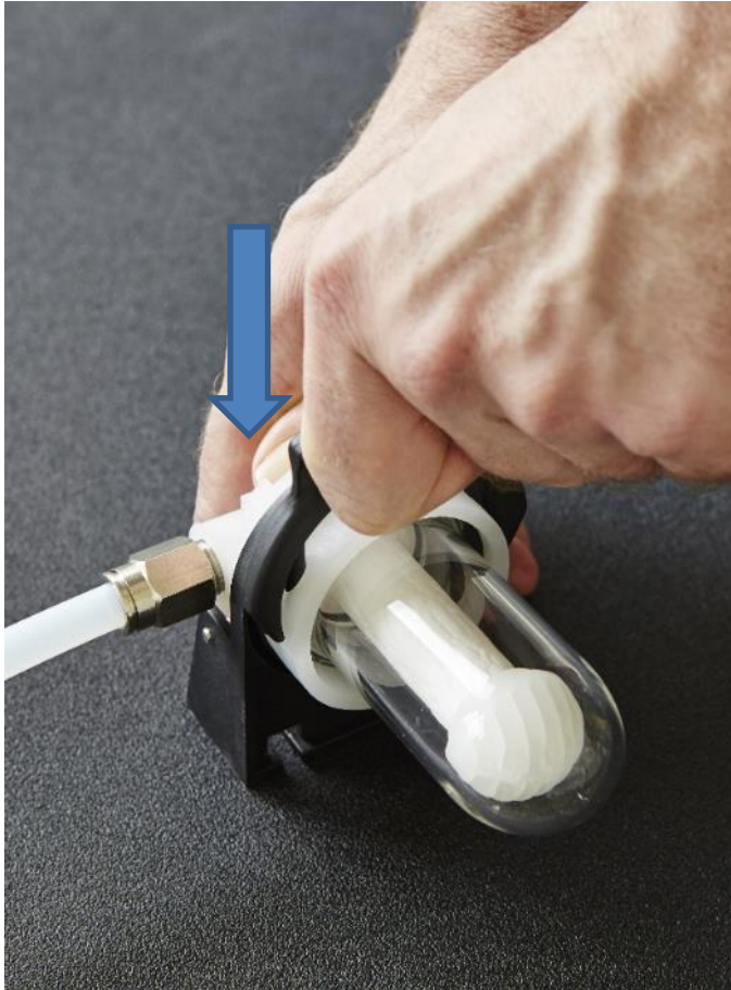
Figure 65 Locking the filter bowl of the coalescing filter
